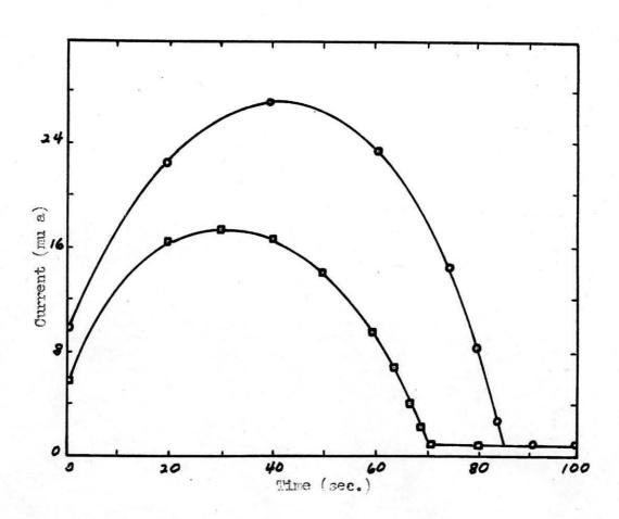
minimum" as the iodide that diffused to the indicator cathode became current limiting. The current minimum would have been zero if only iodine was present; however, due to disproportionation of iodine the minimum was greater.
