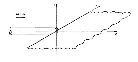
Figure 4.1. Configuration\* for "Flat Plate" Solution,  $\psi''$ . The second solution,  $\psi'^{(2)}$ , may be interpreted then as the solution needed to satisfy the boundary condition of zero flow through the circular
