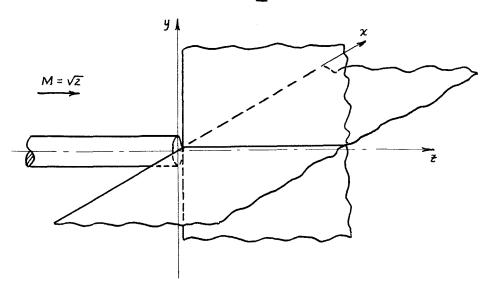
Figure 4.2. Modified "Flat Plate" Configuration: Solution  $\varphi^*$  for  $x \ge 1$ .
