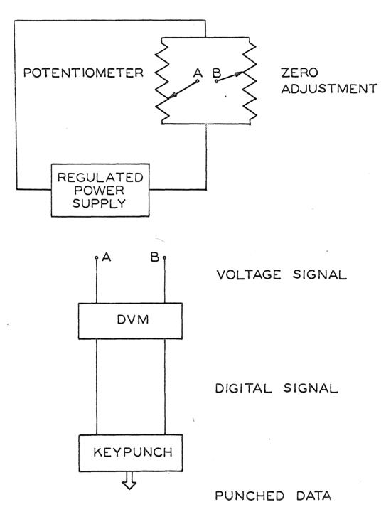
Figure 24. Schematic Diagram of Data Processing Equipment for Raw Film Positions.
