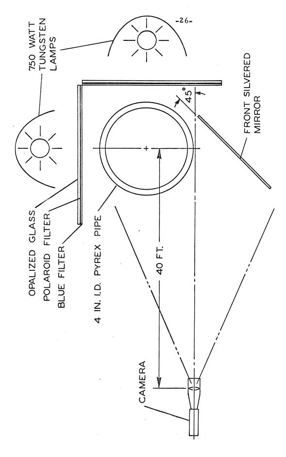
Figure 5. Plan View of the Test Section.
