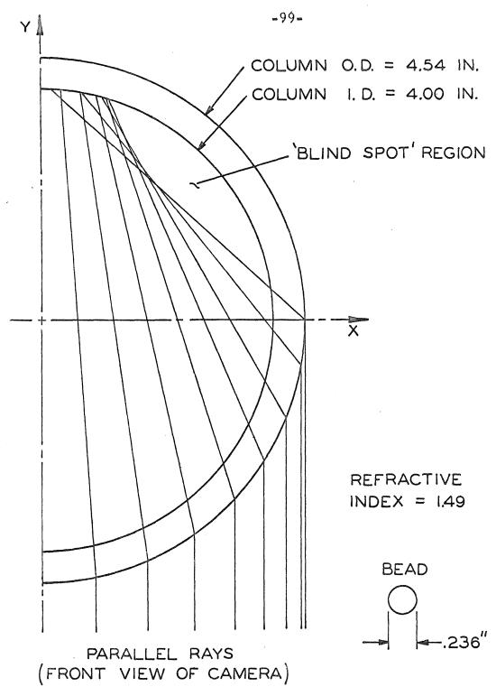
Figure 27. Cross-Sectional View of Column Illustrating Blind Spot Region in Quadrant I. Drawn to Scale.
