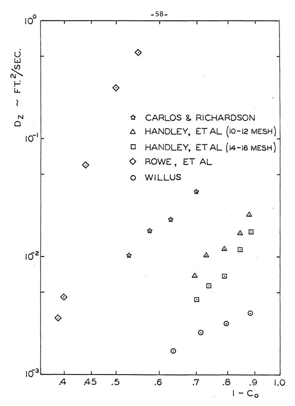
Figure 13. Particle Diffusion Coefficients as a Function of Voidage.
