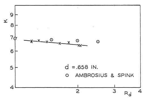
Figure 23. Orifice Coefficient, K, as a Function of Reynolds Number, R<sub>d</sub>, in Tube of 1.94-Inch I. D.
