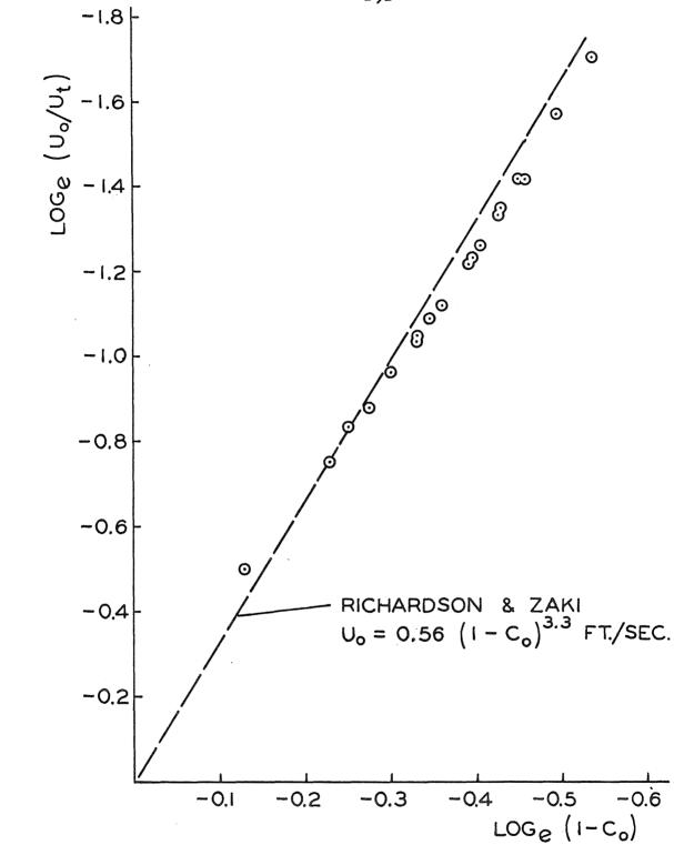
Figure 1. Superficial Fluid Velocity, U, as a Function of Average Particle Voidage, 1-C, at 30°C.
