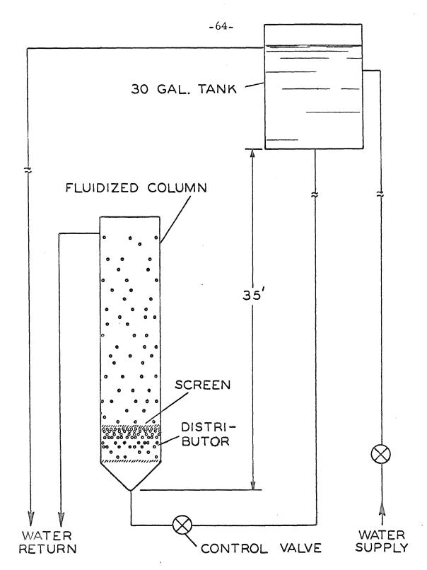
Figure 14. Flow Circuit of the Shallow Bed.
