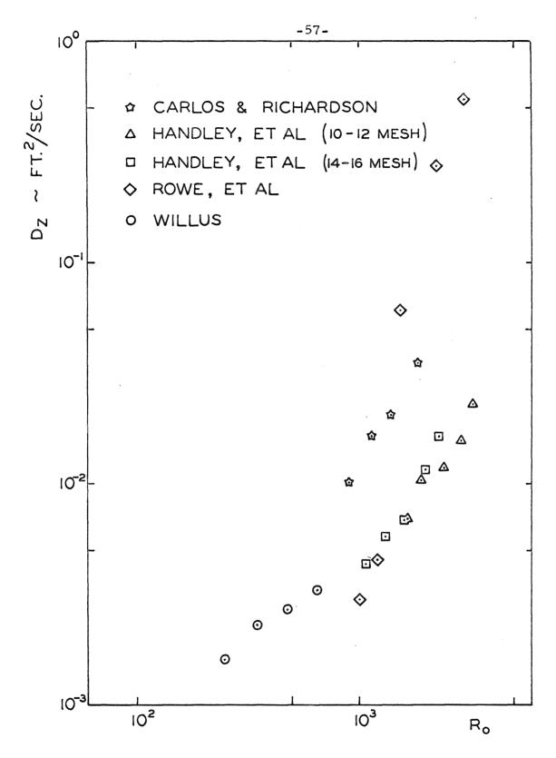
Figure 12. Particle Diffusion Coefficients as a Function of Superficial Reynolds Number Based on Column Diameter.
