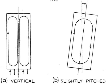
Figure 17. Circulation Patterns in Cylindrical Bed.
