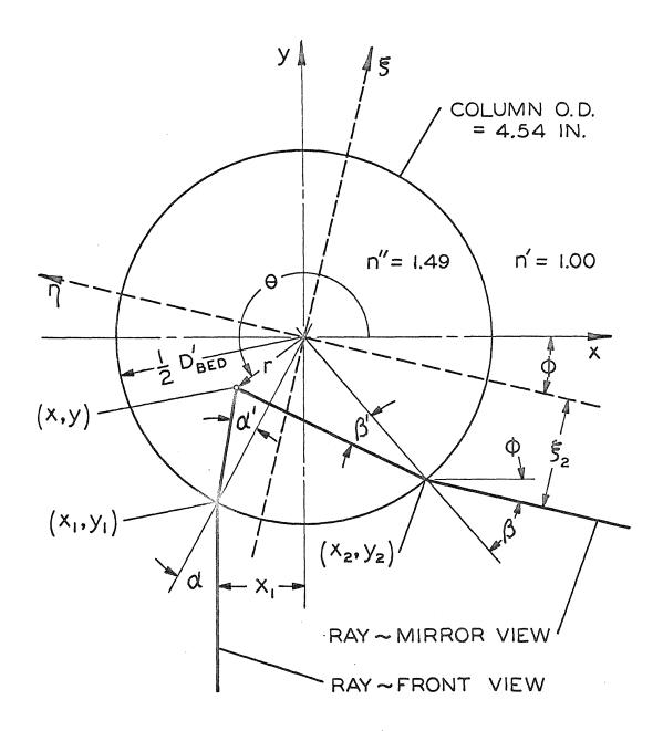
Figure 30. Refracted Rays of a Bead in the Column in the Determination of Polar Position.
