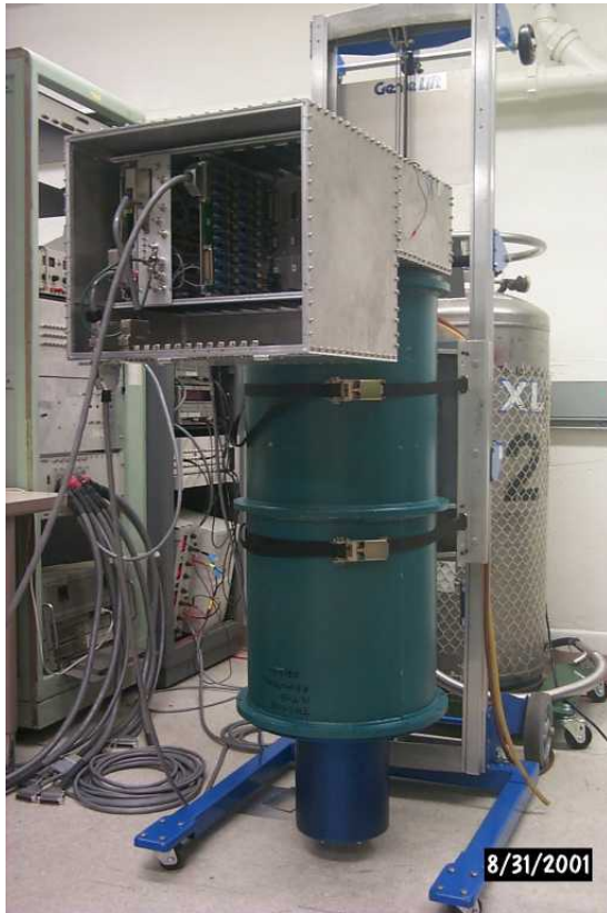
Figure 3.3: The Bolocam dewar in the lab during testing. The electronics box is open and we can see one of the preamp boards. The dewar is downward looking and the window is not visible.
