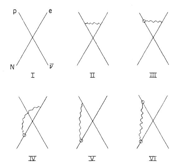
FIGURE 5. FEYNMAN DIAGRAMS FOR NEUTRON DECAY.
