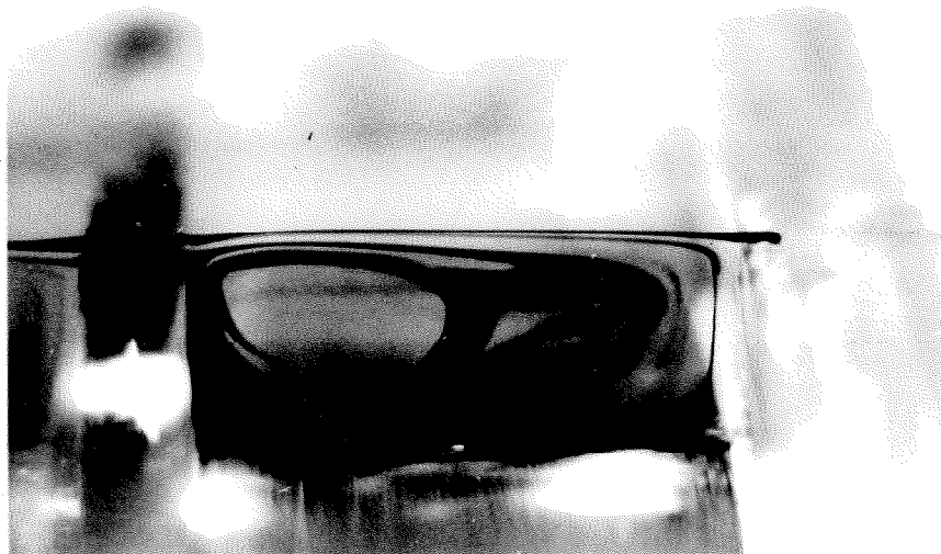
Fig. 37. Photograph of cavity flow. Flow is from right to left. 1/2 inch deep x 1-1/4 inch long cavity, U_{\infty} = 0.25 ft/sec., \epsilon^* = 96.0 .
