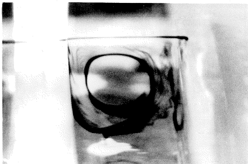
Fig. 43. Photograph of cavity flow showing the laminar oscillation. 1 x 1 in. cavity, U_{\infty} = 0.50 ft/sec., \epsilon^* = 286.4 .
