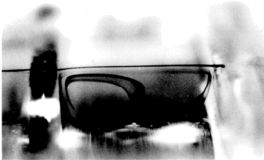
Fig. 38. Photograph of cavity flow. Flow is from right to left. 1/2 inch deep \times 1-1/4 inch long cavity, U_{\infty} = 0.50 ft/sec., \epsilon^* = 143.2 .
