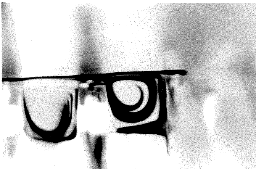
Fig. 21. Photograph of cavity flow. Flow is from right to left. 1/4 \times 1/4 in. cavities, U_{\infty} = 0.50 ft/sec., \epsilon^* = 71.6 .
