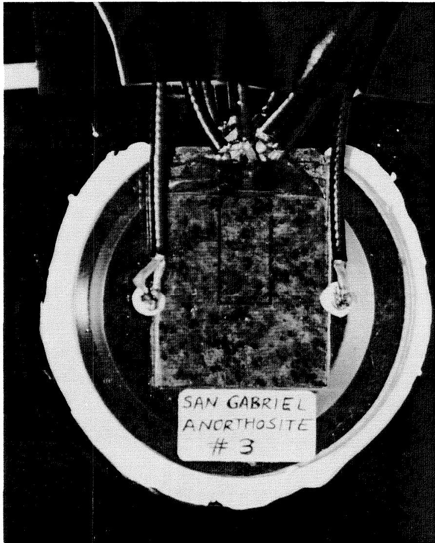
Fig. IV-3. Typical rock sample, with free-surface gauge visible.
