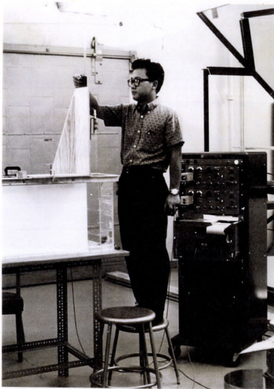
Figure 3-10 Measuring the conductivity profile with the conductivity probe and the Sanborn recorder.
