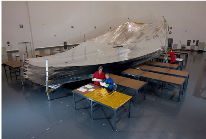
Figure 1.4: Wrinkles on a full-scale sunshield of the James Webb Space Telescope (JWST). The sunshield is undergoing folding and deployment trials to verify its design concept and deployment techniques at Northrop Grumman's Space Technology facility in Redondo Beach, CA (NASA, www.nasa.gov ).
