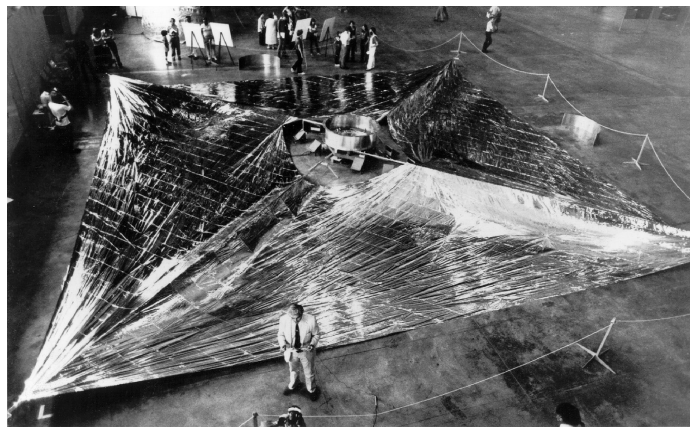
Figure 1.3: Wrinkles on a four quadrant, 20-meter solar sail. The solar sail system is fully deployed during testing at NASA Glenn Research Center's Plum Brook facility in Sandusky, OH (NASA, www.nasa.gov ).
