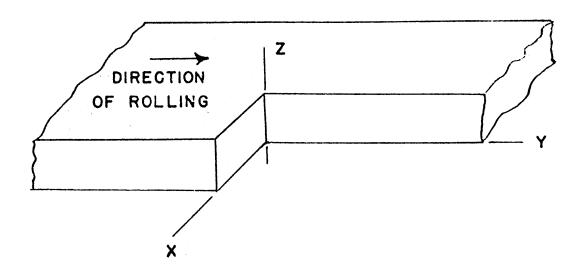
FIGURE 13. Orientation of reference axes in test specimens.
