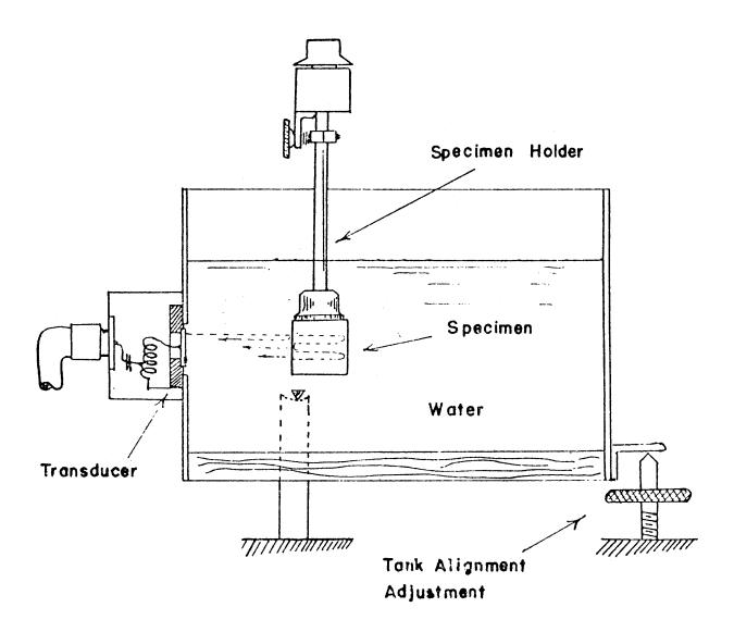
FIGURE 8. Sectional drawing of arrangement of acoustic components.
