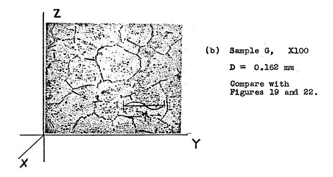
FIGURE 23. Micrographs of Aluminum samples showing structures.
