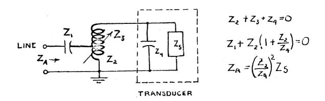
FIGURE 6. HALF-WAVE MATCHING NETWORK.
