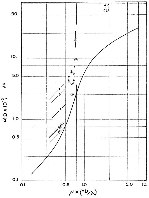
FIGURE 30. Plot of observed attenuations versus mean grain diameter on the dimensionless scales. The leaters indicate the direction of propagation. The encircled points are for duralumin, the others for aluminum. The solid curve is the derived relation shown in rigure 3.
