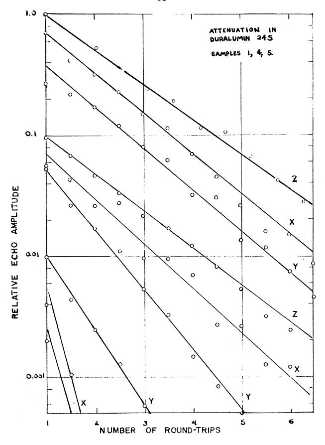
FIGURE 14. Unreduced data for duralumin samples.
