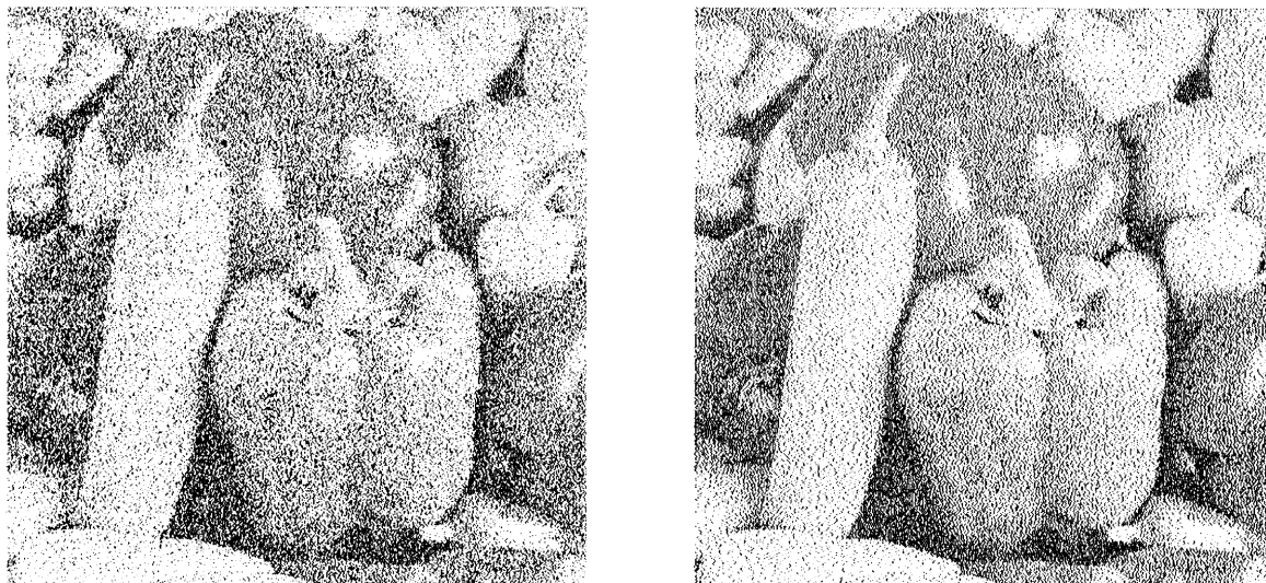
Figure 3.22: Left: Result of first adding zero mean, Gaussian white noise n before passing each horizontal scan line of the image from Figure 3.4 through an IFC using the design rule from the last section. Right: Same as the image on the left, but using less noise. See text for details.
