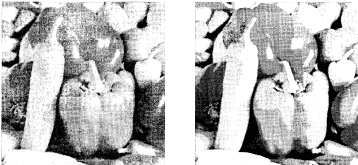
Figure 3.15: Left : Result of passing the quantized image from Figure 3.14 through a spatiotemporal linear filter designed assuming both a temporal oversampling ratio and a spatial oversampling ratio of four. This reduces the power of the quantization error in the resulting image by a total factor of sixteen times. Right : Result of passing the quantized image from Figure 3.7 through the same filter, illustrating that signal-dependent quantization error cannot be significantly reduced with linear filtering.
