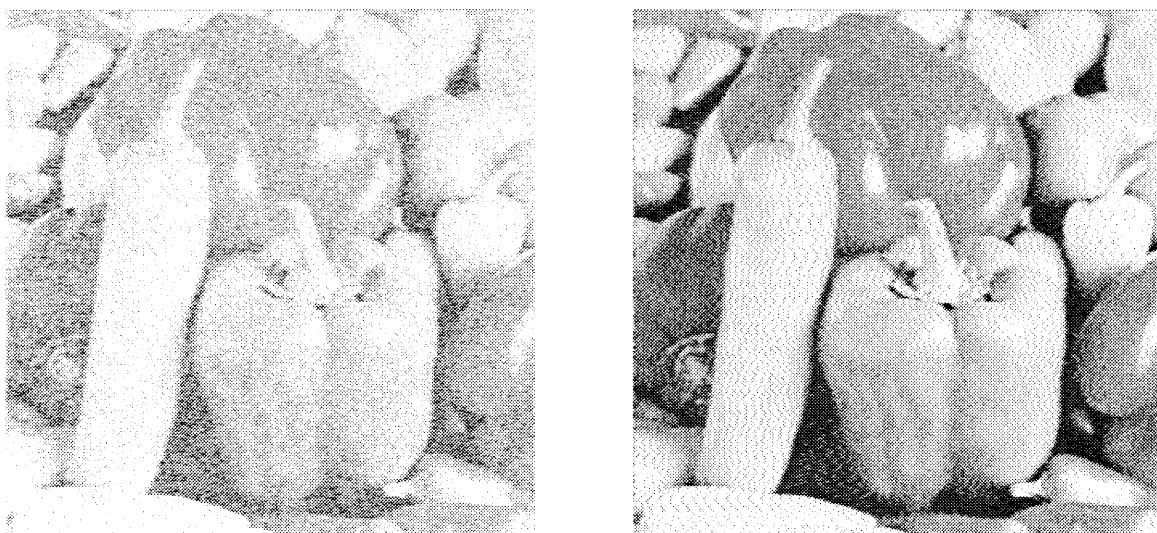
Figure 3.23: Left: Result of temporally integrating each horizontal scan line from the IFC encoded image on the right in Figure 3.22 with a low pass filter whose cutoff frequency is at the bandwidth of s , thus reducing the power of quantization error. Right: Result of doing the same with the image from Figure 3.21, illustrating that a linear filter provides little reduction for signal dependent quantization error.
