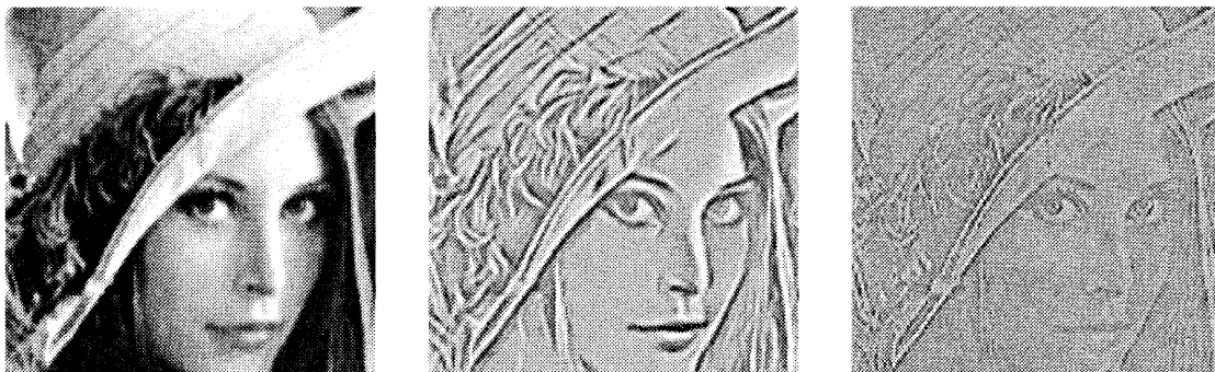
Figure 2.24: Left: A 128 \times 128 section of the IEEE standard image, “Lena,” which was not used in training. Center: Result of reconstructing the image from simulated simple cell responses (see text for explanation). Right: The normalized, smoothed and whitened image, shown for comparison.
