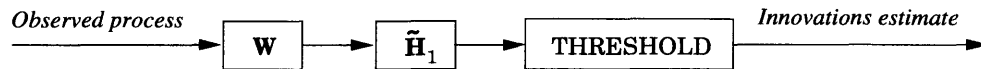
Figure 2.15: The innovations estimator of the third stage. The generalized matched filter is a whitening filter followed by a postwhitened matched filter.
