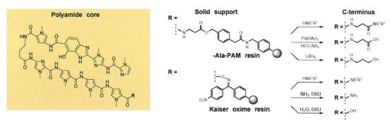
**Figure 1.8** (Left) Oligomer synthesized using solid phase methodology. (Center) Resin systems used for polyamide synthesis. (Right) Cleavage conditions for modulating the chemical functionality at the C-terminus of a polyamide.
