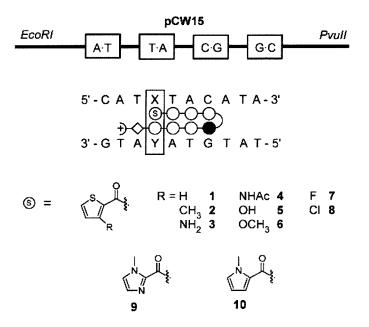
**Figure 4.2** (top) pCW15 plasmid design. (bottom) Ball and stick model of hairpin polyamides varying the N-terminal residue. Shaded and non-shaded circles represent imidazole and pyrrole residues, respectively. A circle containing an S denotes an N-terminal thiophene (R = 1-8) residue.
