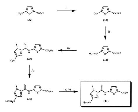
**Figure 2.8** Synthesis of **Tp** containing dimers. (i) H<sub>2</sub>SO<sub>4</sub>, MeOH, Reflux; (ii) SnCl<sub>2</sub>.2H<sub>2</sub>O, 95% EtOH, 37% HCl, 35°C; (iii) NO<sub>2</sub>-Im-COCCl<sub>3</sub>, EtOAc, 35°C; (iv) H<sub>2</sub> Pd/C, EtOAc, 500psi, R.T.; (v) (BOC)<sub>2</sub>O, DIEA, DMF, 60°C; (vi) 1N NaOH, MeOH, 60°C.
