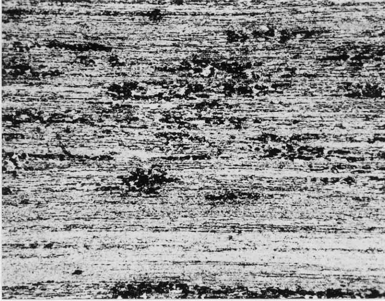
Fig. 59. 25 per cent chromium-iron, cold rolled 99 per cent, aged 910.5 hours at 540°C. 195 VHN. Mechanical polish. Glyceregia etch. 500X.
