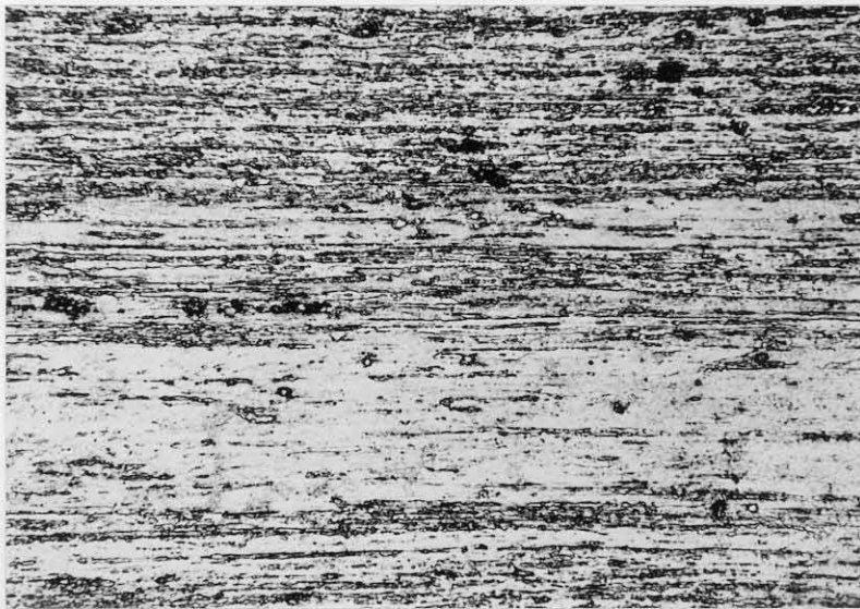
Fig. 58. 25 per cent chromium-iron, cold rolled 99 per cent, aged 100 hours at 540°C. 272 VHN. Mechanical polish. Glyceregia etch. 500X.
