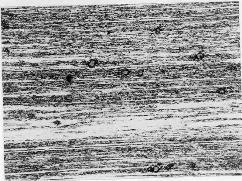
Fig. 61. 34 per cent chromium-iron, cold rolled 99 per cent, aged 900 hours at 456°C. 438 VHN. Mechanical polish. Glyceregia etch. 500X.
