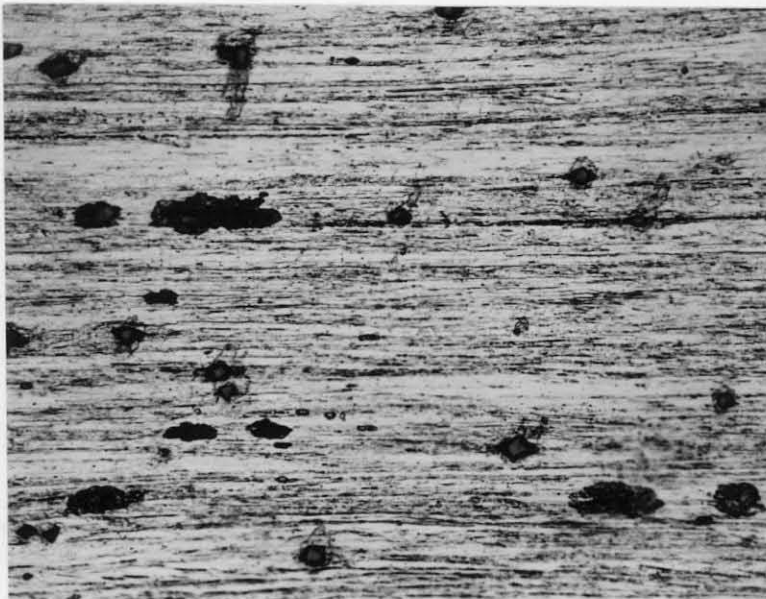
Fig. 66. 42 per cent chromium-iron, cold rolled 99 per cent, aged 98.8 hours at 540°C. 373 VHN. Mechanical polish. Glyceregia etch. 500X.
