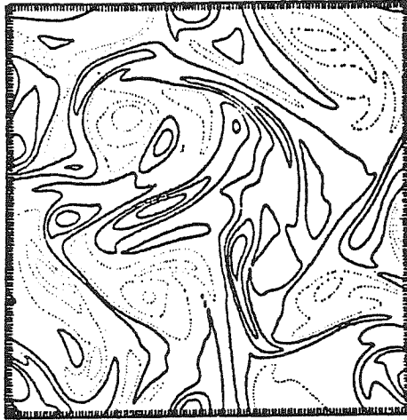
Fig. 2: Vorticity field obtained at t=2 by Herring et al. [16] with \nu=0.005 and Re=138 .
