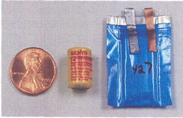
Figure A-11: Lithium polymer battery in comparison to Sanyo N50-AAA battery
