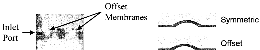
Figure 5-15: Offset membrane location (to the left) to improve sealing. The blue dye illustrates the resulting dead volume.
