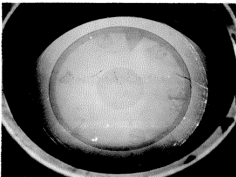
e. Stationary with 130.4 psig oil pressure. Average seal face pressure 68.7 psi.
