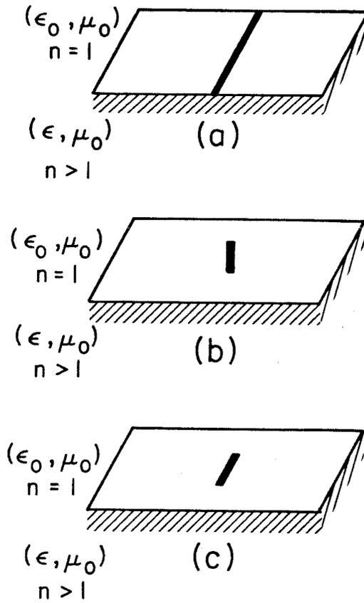
Fig. 1. Three interfacial radiating sources: (a) infinitely long line source, (b) infinitesimal vertical dipole, and (c) infinitesimal horizontal dipole.
