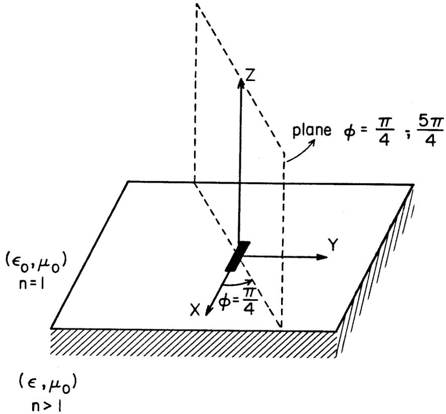
Fig. 15a. The mathematical plane normal to the interface and bisecting the dipole with angle  $\phi = \frac{\pi}{4}$ .
