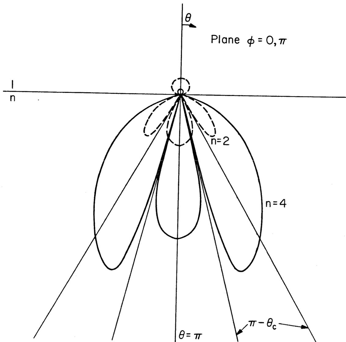
Fig. 14b. Radiation pattern of the horizontal dipole in the mathematical plane shown in Fig. 14a. For any value of  $n$ , there are nulls along the interface and along the angle  $\theta = \pi - \theta_c$  in the plane  $\phi = 0, \pi$ . Here  $\sin \theta_c = \frac{1}{4}$  (continuous line) and  $\sin \theta_c = \frac{1}{2}$  (broken line).
