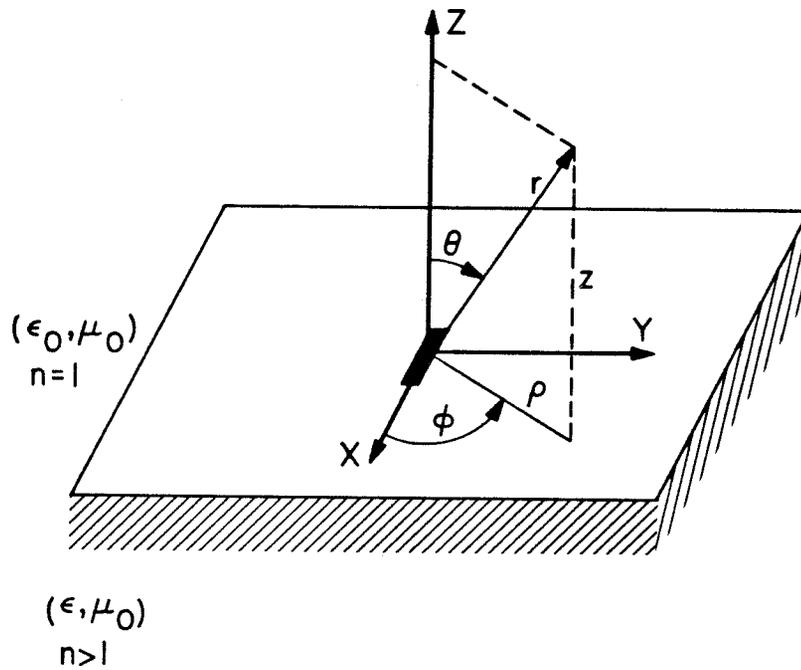
Fig. 13. The infinitesimal electric dipole is located on the interface and is directed parallel to x axis. In the upper half-space ( $z > 0$ ) the dielectric constant is  $\epsilon_0$  and in the lower half-space ( $z < 0$ ) the dielectric constant is  $\epsilon$  which is greater than  $\epsilon_0$ .
