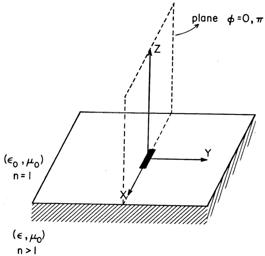
Fig. 14a. The mathematical plane normal to the interface and containing the dipole (plane  $\phi = 0, \pi$ ).
