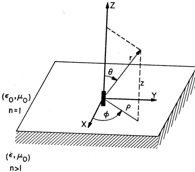
Fig. 9. The infinitesimal electric dipole is located on the interface and is normal to it. The dielectric constant of the upper half-space ( $z > 0$ ) is  $\epsilon_0$  and that of the subsurface region ( $z < 0$ ) is  $\epsilon$  which is greater than  $\epsilon_0$ .
