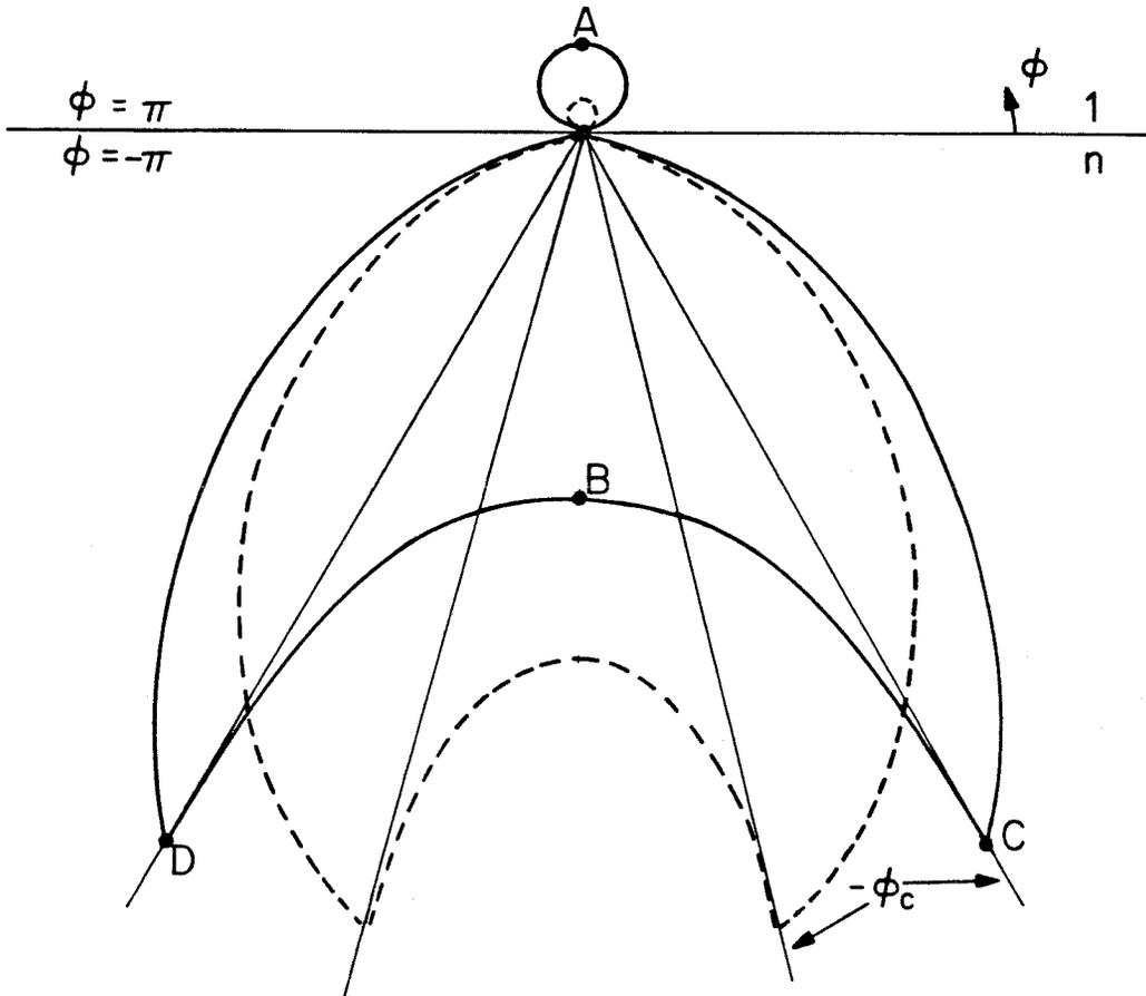
Fig. 3. Radiation patterns for  $n = 2$  (continuous line) and  $n = 4$  (broken line). As the index of refraction  $n$  of subsurface region increases, the lobe in the upper half-space shrinks, the dihedral angle between the two (Cerenkov) peaks D and C decreases, and the point B moves downward. For all values of  $n > 1$ , there is a broad null along the interface. Here  $\cos \phi_c = 1/2$  (continuous line) and  $\cos \phi_c = 1/4$  (broken line).
