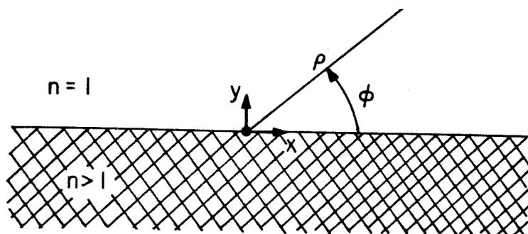
Fig. 2. Line source lies along  $z$  axis. In the upper half-space ( $y > 0$ ) the index of refraction  $n$  is equal to 1, and in the lower half-space ( $y < 0$ )  $n$  is greater than 1.
