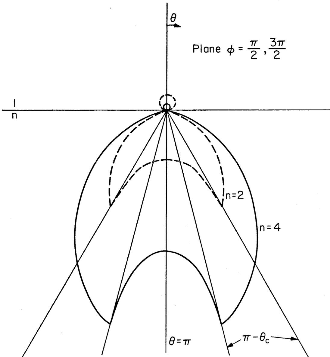
Fig. 16b. Radiation pattern of the horizontal dipole in the mathematical plane shown in Fig. 16a for  $n=4$  (continuous line) and  $n=2$  (broken line).
