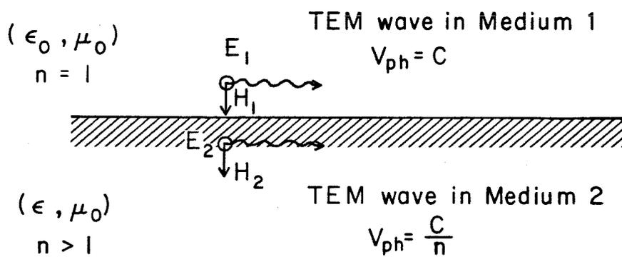
Fig. 8. Impossibility of matching two TEM waves with nonzero amplitudes and different phase velocities.
