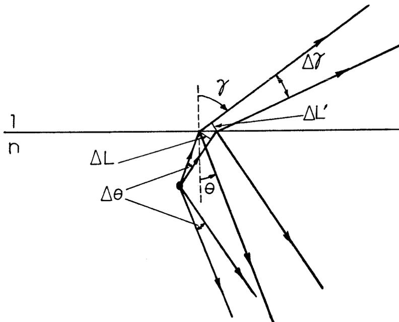
Fig. 7. Ray diagram for case of source a little below interface.
