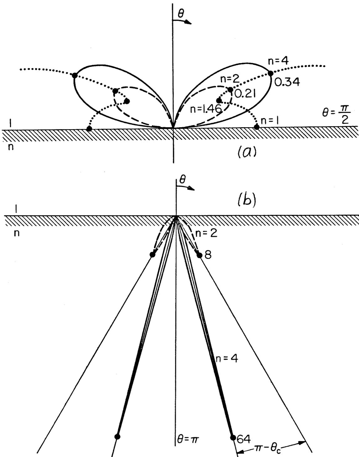
Fig. 10. Radiation pattern of the vertical dipole of Fig. 9 (a) in the upper half-space, (b) in the lower half-space for  $n=4$  (continuous line) and  $n=2$  (broken line). The dotted curve ( $L$ ) is the locus of the maxima of the pattern in the upper half-space, as  $n$  increases from one to infinity. Note that the scale in Fig.10(a) is different from that of Fig. 10(b).
