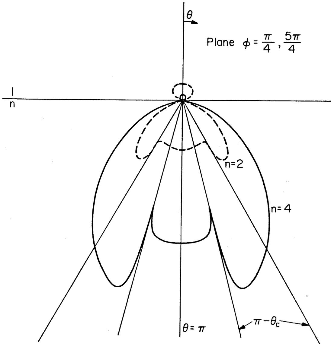
Fig. 15b. Radiation pattern of the horizontal dipole in the mathematical plane shown in Fig. 15a for  $n=4$  (continuous line) and  $n=2$  (broken line).
