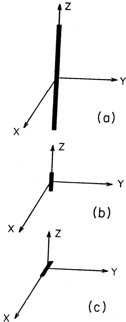
Fig. 18. (a) infinitely long line source in free-space, (b) and (c) infinitesimal electric dipole in free-space directed parallel to the z and x axes respectively.
