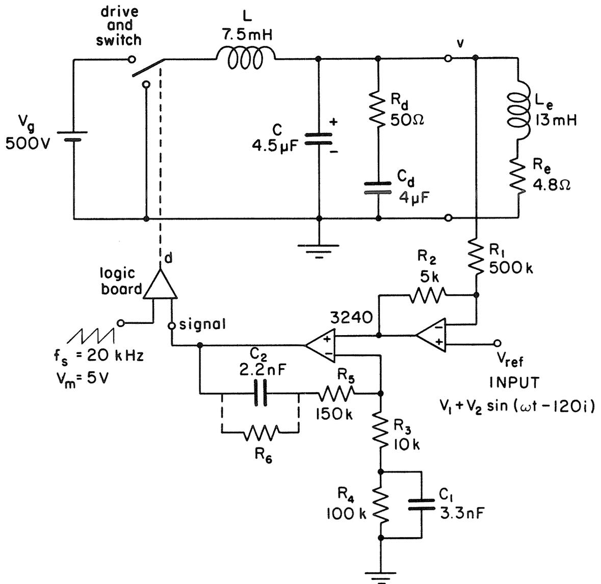
Fig. 13.7 Complete closed-loop schematic of one phase of the amplifier.
