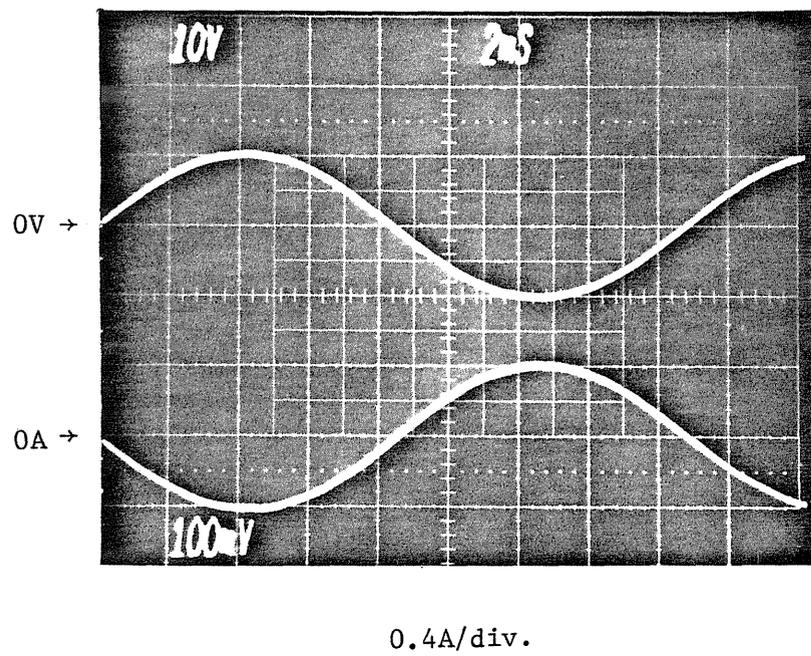
Fig. 8.11 Oscillogram of the ac voltage and current of the battery charger ( $R_{out} = 25\Omega$ ).
