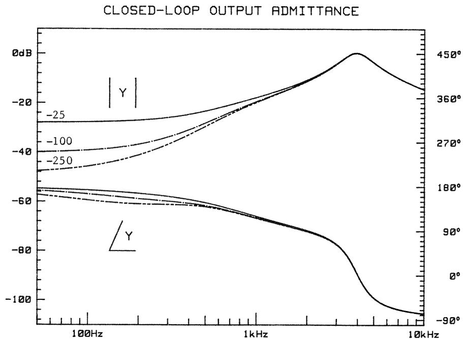
Fig. 8.10 Families of output admittance transfer functions. (a) Battery charger: Cases of  $25\Omega$ ,  $100\Omega$ , and  $250\Omega$ , (b) battery discharger: Cases of  $-25\Omega$ ,  $-100\Omega$ , and  $-250\Omega$ . Zero dB corresponds to  $1\Omega$  (1 mho).
