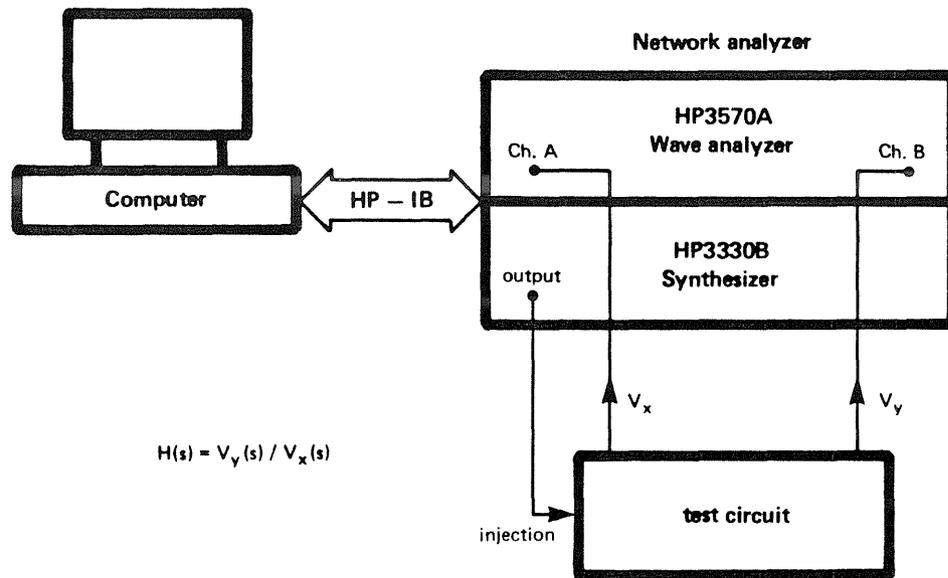
Fig. 3.3 Automated frequency response measurement system composed of frequency synthesizer, wave analyzer, and computer as controller.
