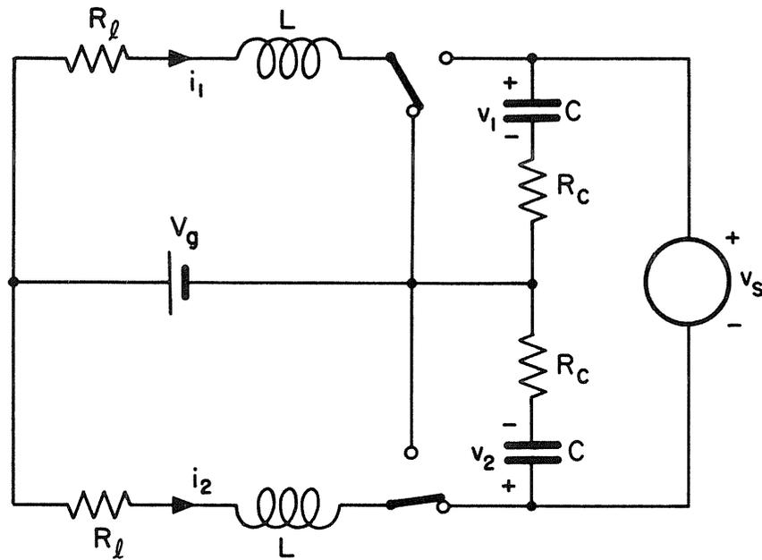
Fig. 8.3 Boost amplifier example with inductor and capacitor resistive parasitics.
