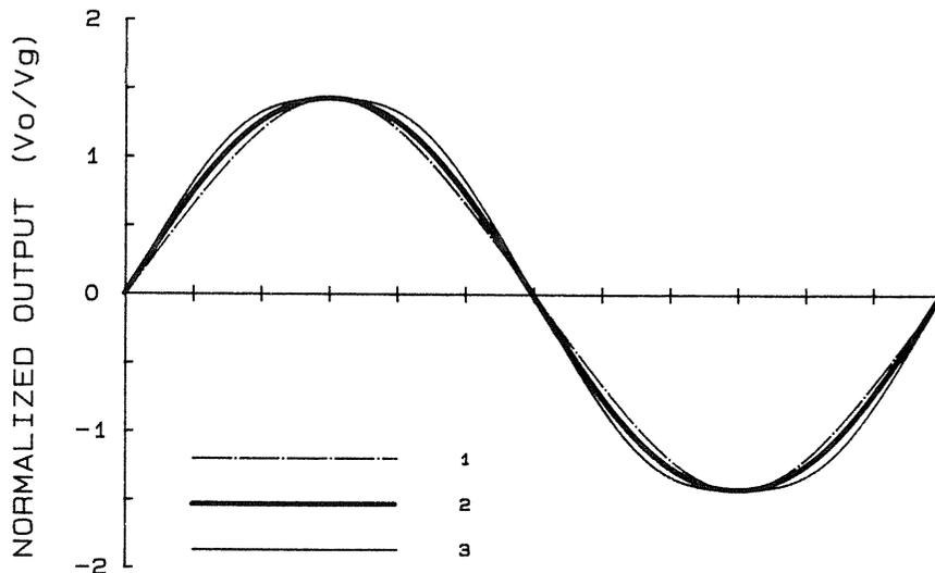
Fig. 7.5 Low frequency sine waves generated by nonlinear amplifiers. (1) Ideal (all), (2) linearized Ćuk, and (3) linearized boost and buck-boost.
