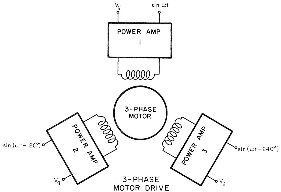
Fig. 12.1 Three-phase motor drive employing three regulated switching power amplifiers.
