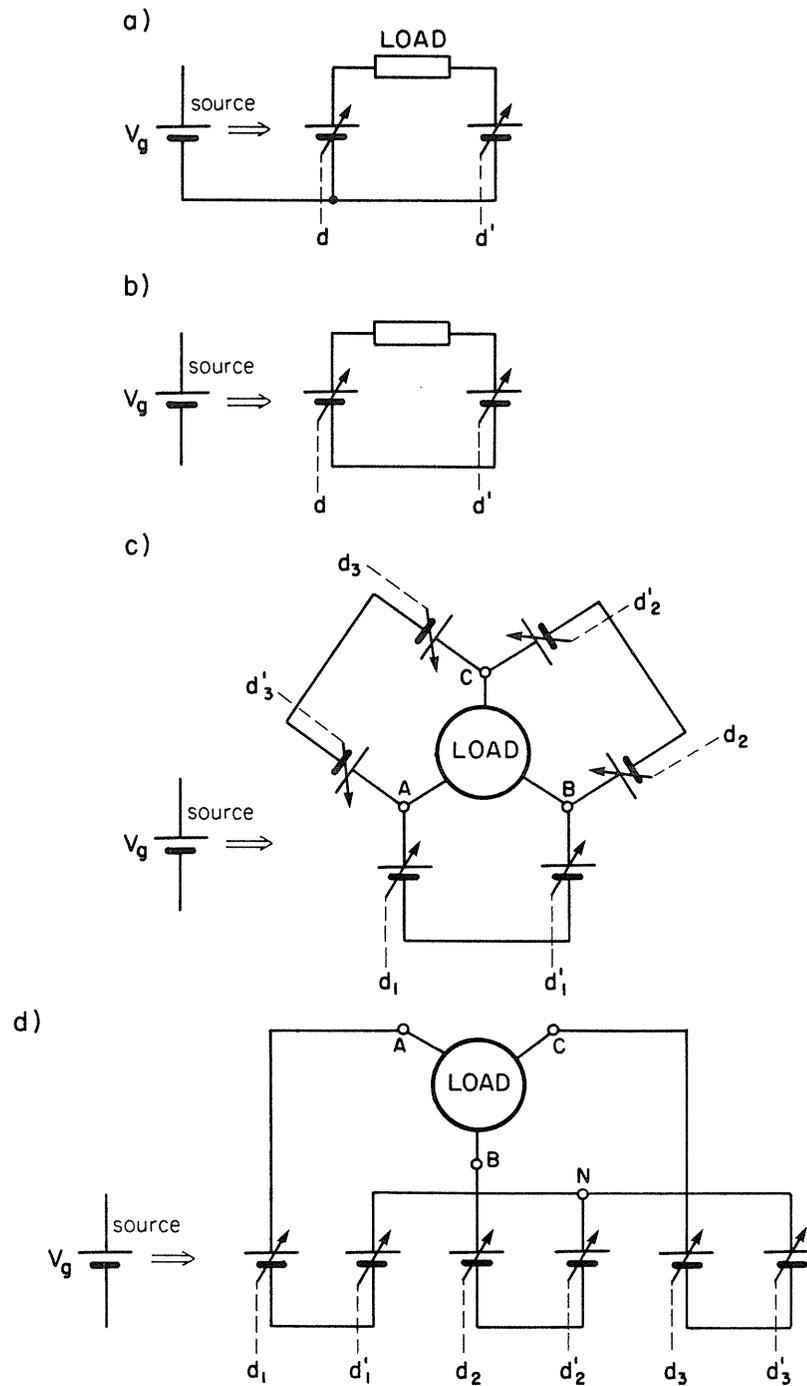
Fig. 12.2 General three-phase connection: (a) a single-phase power amplifier, (b) isolated single-phase inverter, (c) delta connection of inverters, (d) star connection of inverters.
