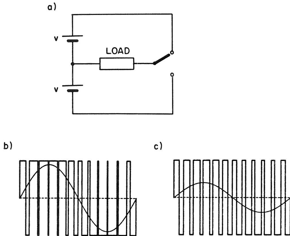
Fig. 6.3 Pulse Width Modulation technique. (a) The hardware, (b) high-level output, (c) low-level output.
