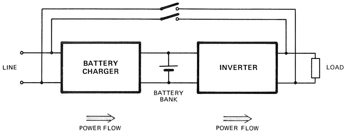
Fig. 5.1 A conventional ac Uninterruptible Power Supply.
