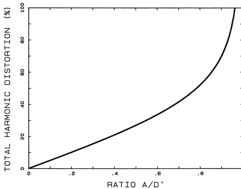
Fig. 12.9 Total harmonic distortion for boost, buck-boost, and Ćuk three-phase amplifiers.
