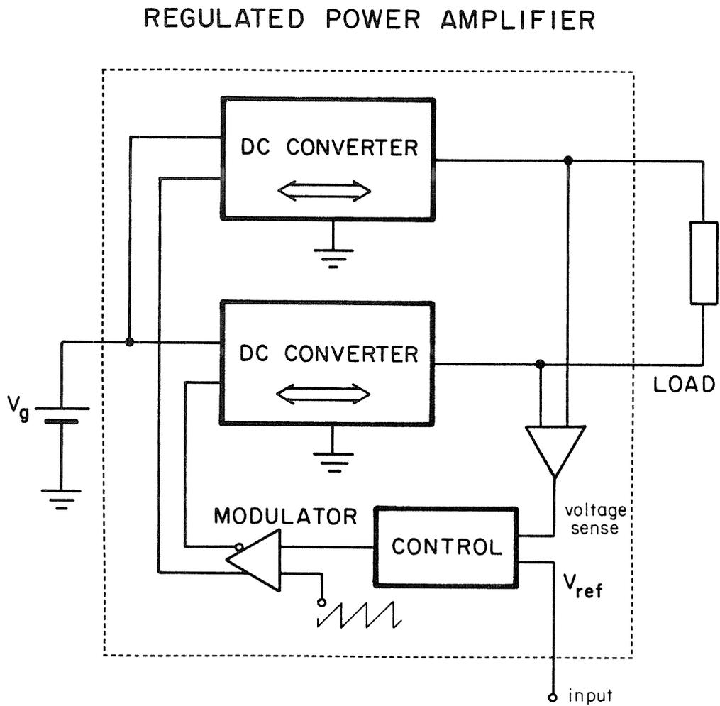
Fig. 7.2 Output voltage regulation of a push-pull amplifier. The sensed output voltage is compared with the reference voltage and the error is kept minimal by the feedback loop.
