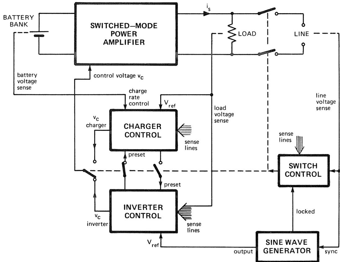
Fig. 9.1 The complete single-unit uninterruptible power supply. Switches are set for inverter mode.
