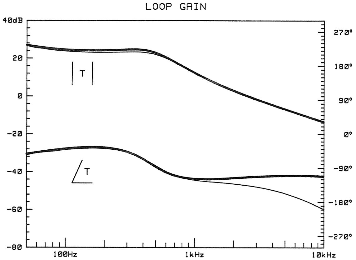
Fig. 7.11 Loop gain. Thick lines: Prediction. Thin lines: Measurement.
