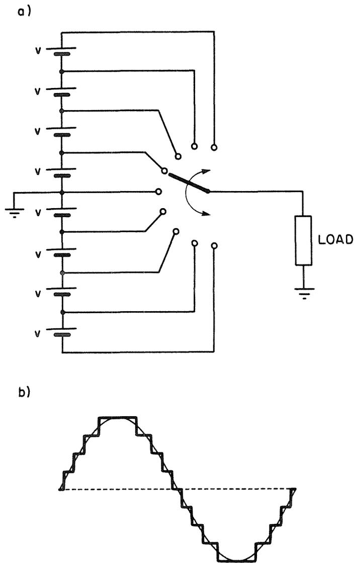
Fig. 6.1 Ac generation with synthesis method. (a) The hardware, (b) output waveform.
