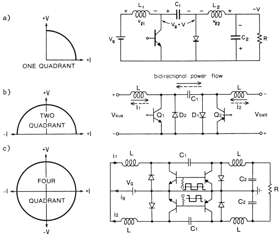
Fig. 6.8 Generalization of dc-to-dc converters. (a) Single-quadrant, (b) current-bidirectional (2-quadrant), (c) push-pull amplifier (4-quadrant).
