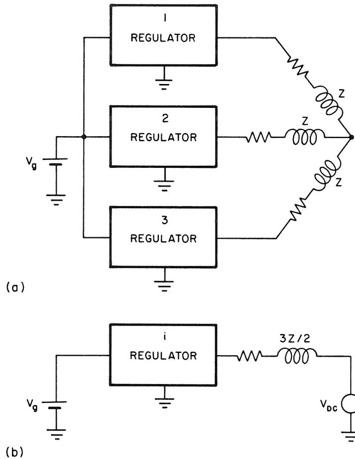
Fig. 13.5 (a) Model of the amplifier and the motor. (b) Simplified model for one phase.
