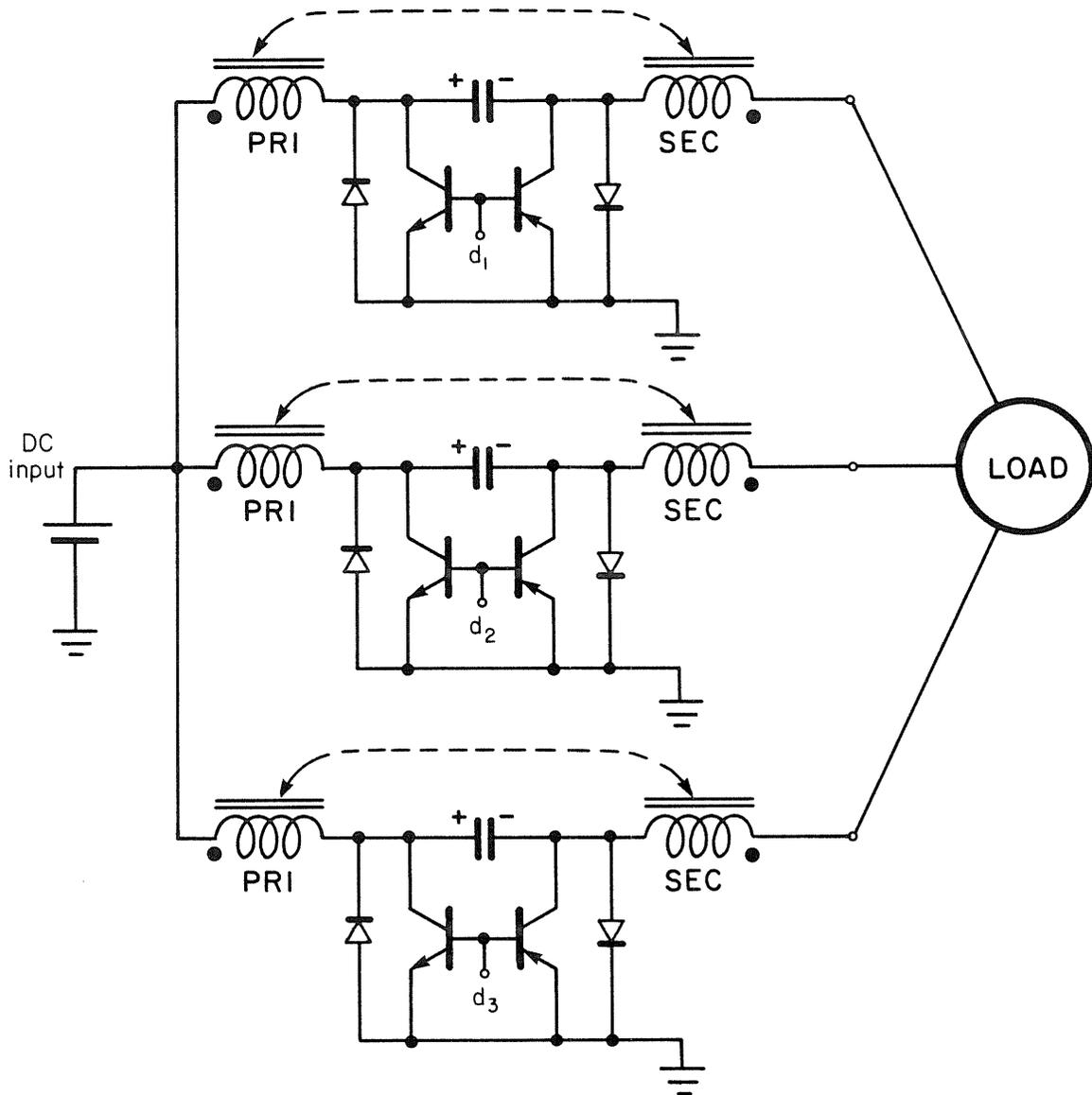
Fig. 12.6 Three-phase switching amplifier employing three Ćuk converters. The  $d_1$ ,  $d_2$ , and  $d_3$  are connected to the modulators.
