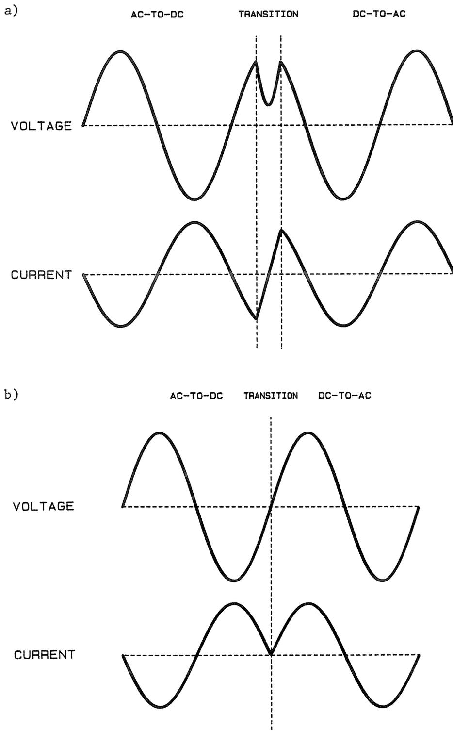
Fig. 9.4 Transition from charger to inverter mode. (a) Worst case, (b) an easy case!
