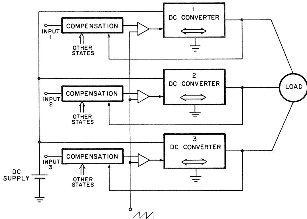
Fig. 13.3 General form of output voltage regulation of the three-phase amplifier.
