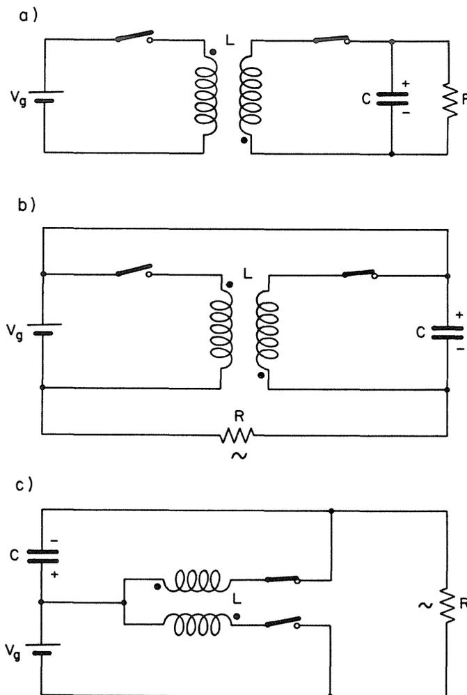
Fig. 6.6 Buck-boost differential amplifier (a) isolated converter, (b) output in series with input, (c) the same as (b), but drawn differently.
