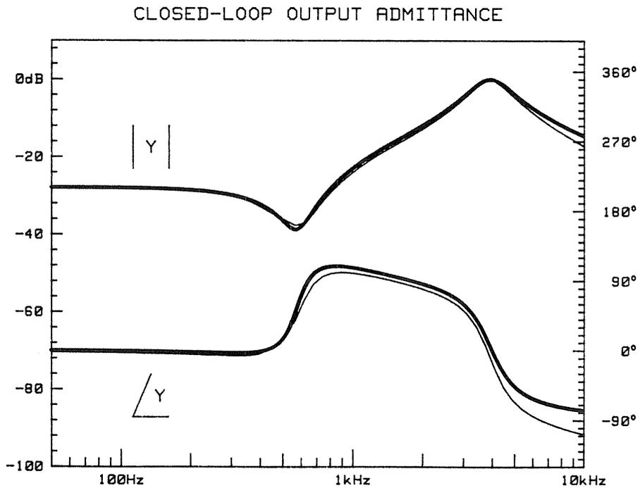
Fig. 8.9 Output admittance, (a) theoretical, open-loop; (b) theoretical (thick lines) and measurement (thin lines) results for closed-loop admittance of  $25\Omega$  nominal. Zero dB corresponds to  $1\Omega$  (1 mho).
