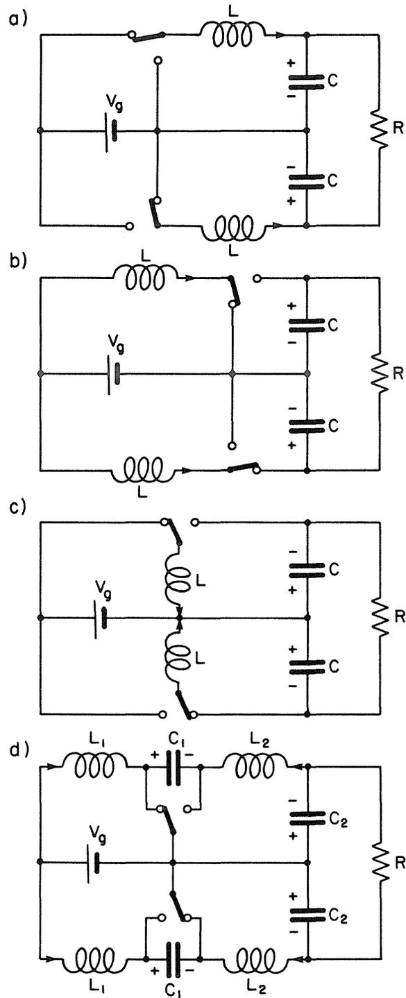
Fig. 7.1 Four push-pull switching amplifiers each consisting of two current-bidirectional converters.
