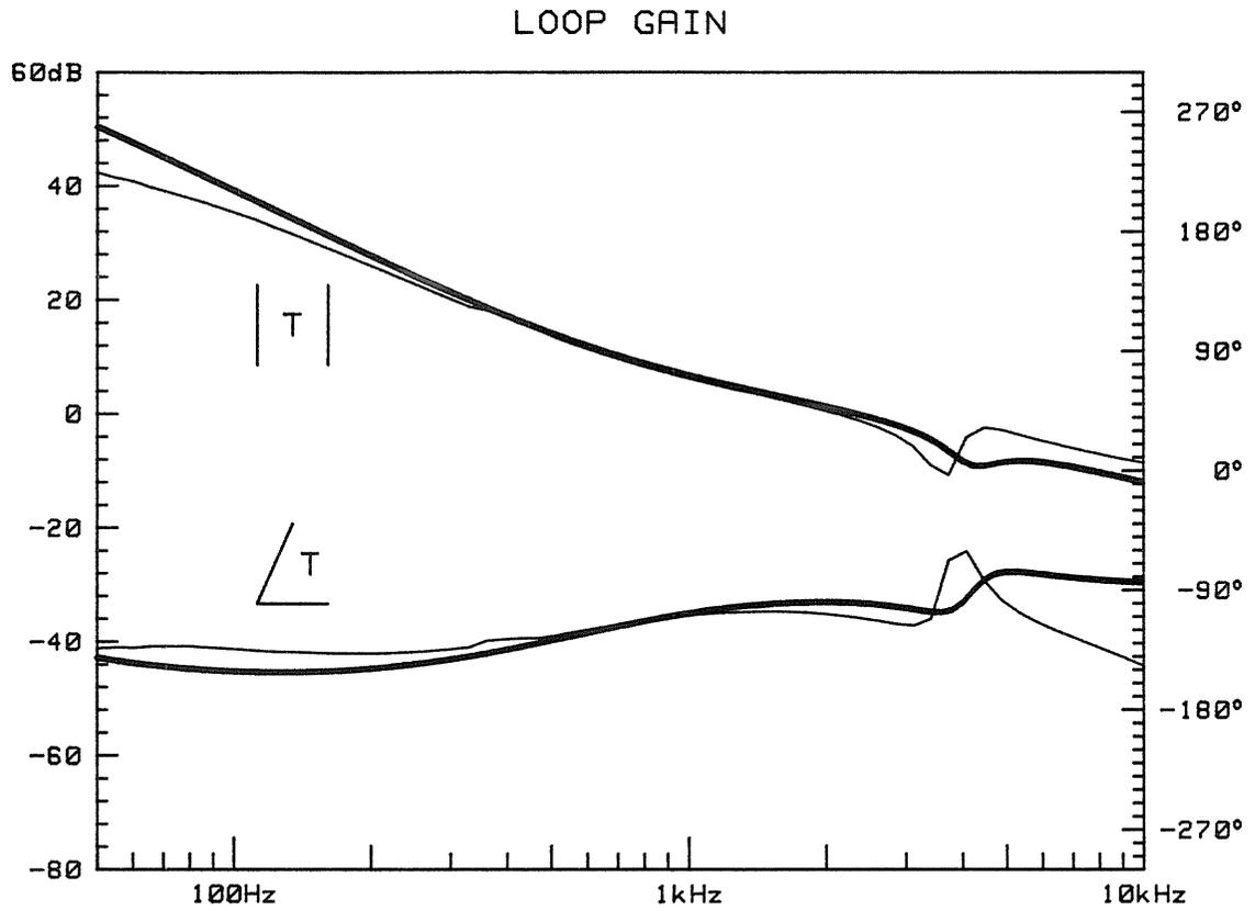
Fig. 8.8 Predicted and measured loop gain of the battery charger.
