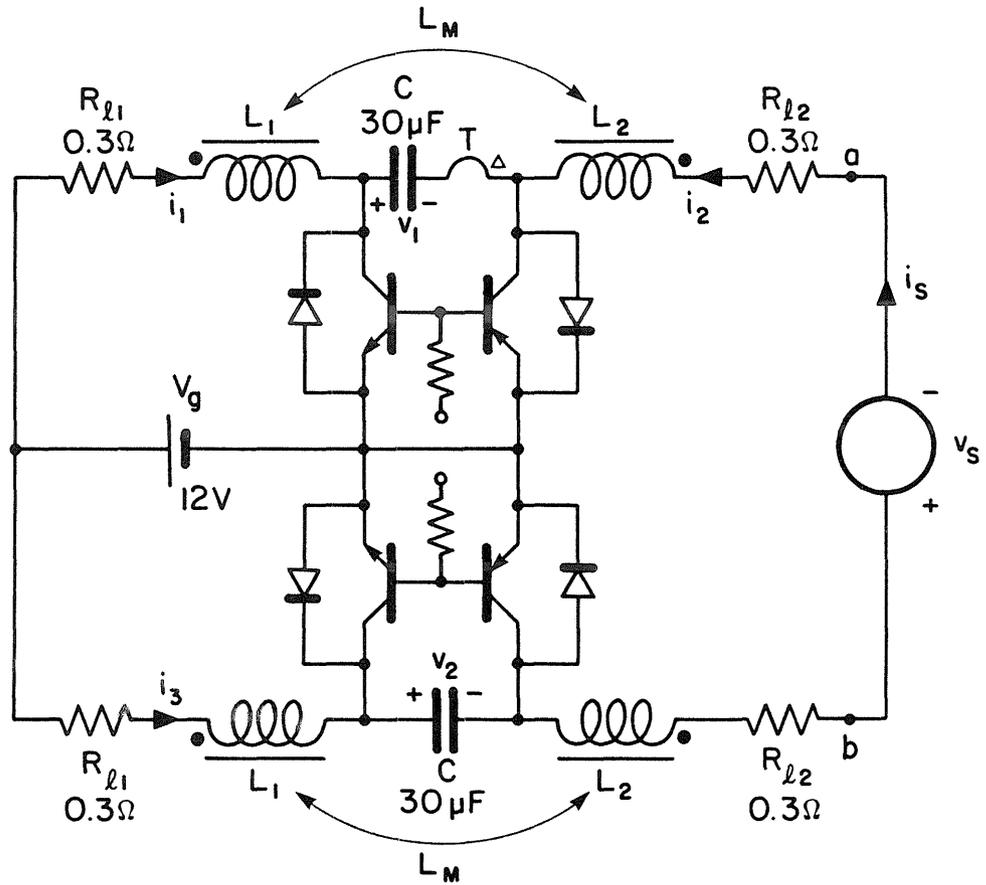
Fig. 8.4 Experimental Ćuk battery charger. The current transformer  $T$  is used to sense  $i_1$  and  $i_2$ .
