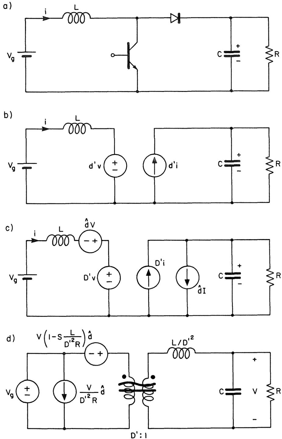
Fig. 2.1 Equivalent circuit approach (a) ideal boost converter, (b) the averaged model, (c) perturbed and linearized model, (d) and the final form.
