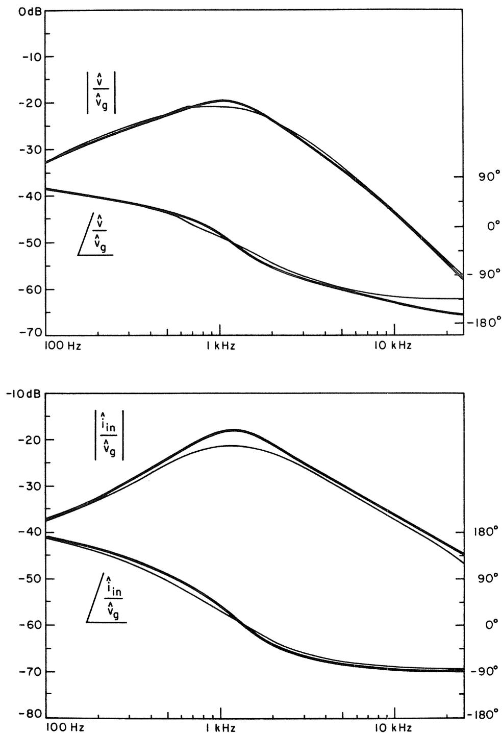
Fig. 3.5 Comparison of the prediction (thick lines) and the measurement (thin lines) result on buck regulator of Fig. 3.4. (a) Closed-loop audio susceptibility, (b) closed-loop input admittance. Notice the phase-shift at low frequencies which denotes a negative impedance.
