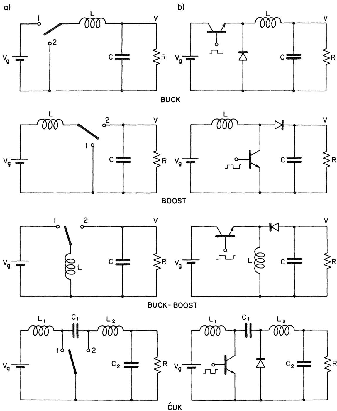
Fig. 1.1 Four common switching dc-to-dc converters: (a) topological configuration (b) bipolar transistor implementation of the switch  $S$ .
