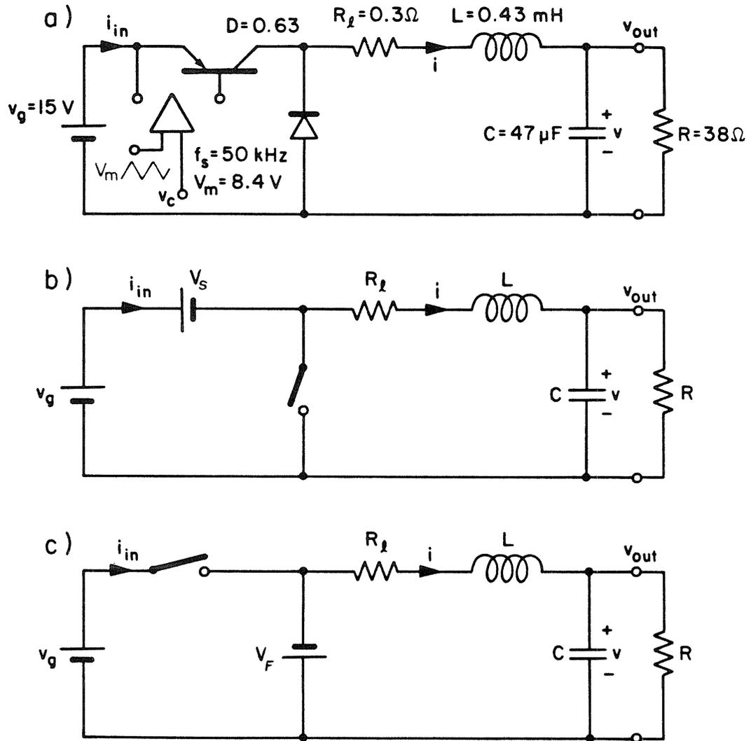
Fig. 3.1 Use of generalized state-space averaging method. (a) The actual circuit, resultant circuit when transistor is (b) on, and (c) off.
