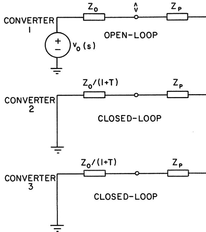
Fig. 13.9 Load impedance for one converter with the other converters regulated.
