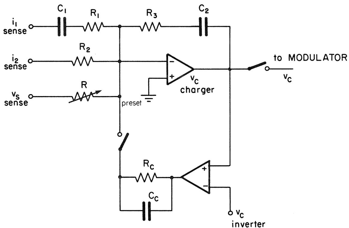
Fig. 9.3 Active circuit to preset the correct voltage in the integrator capacitor of charger controller. (States of the switches are the same as those of Fig. 9.1).
