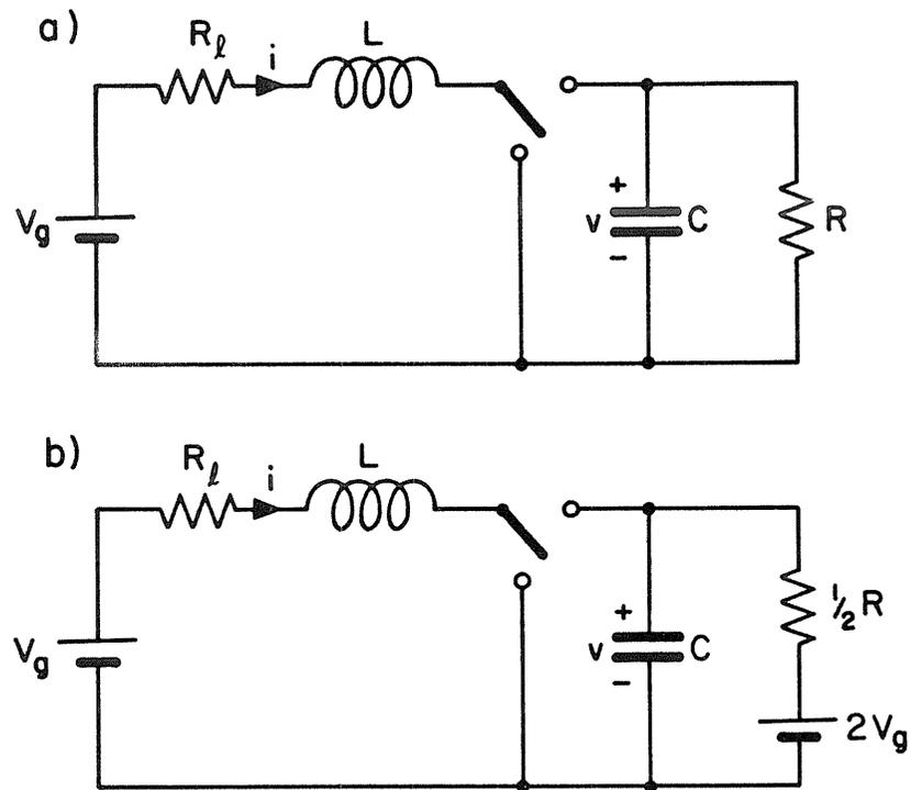
Fig. 7.7 Analysis of amplifier considering one converter. (a) Wrong conditions, (b) correct conditions.
