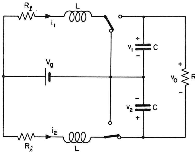
Fig. 7.3 Boost amplifier example with parasitics inductor resistances included.
