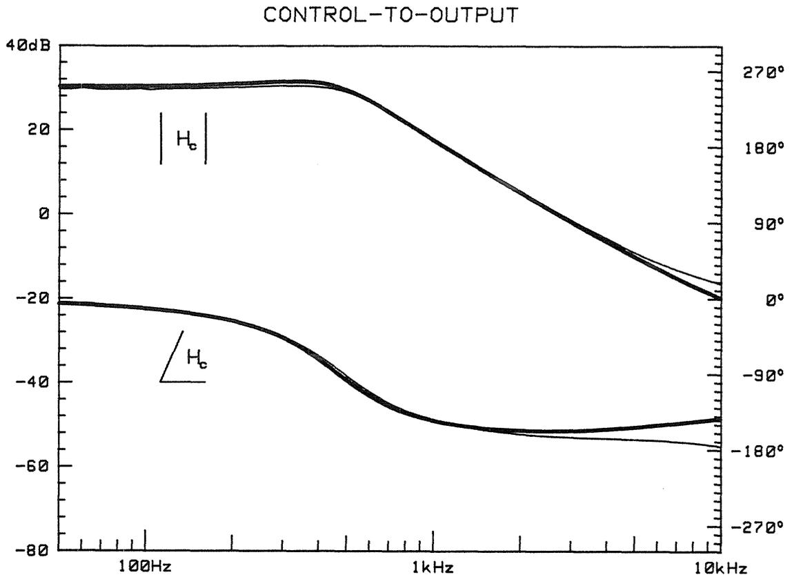
Fig. 7.9 Predicted (thick lines) and measured (thin lines) control-to-output transfer function of the Cuk amplifier.
