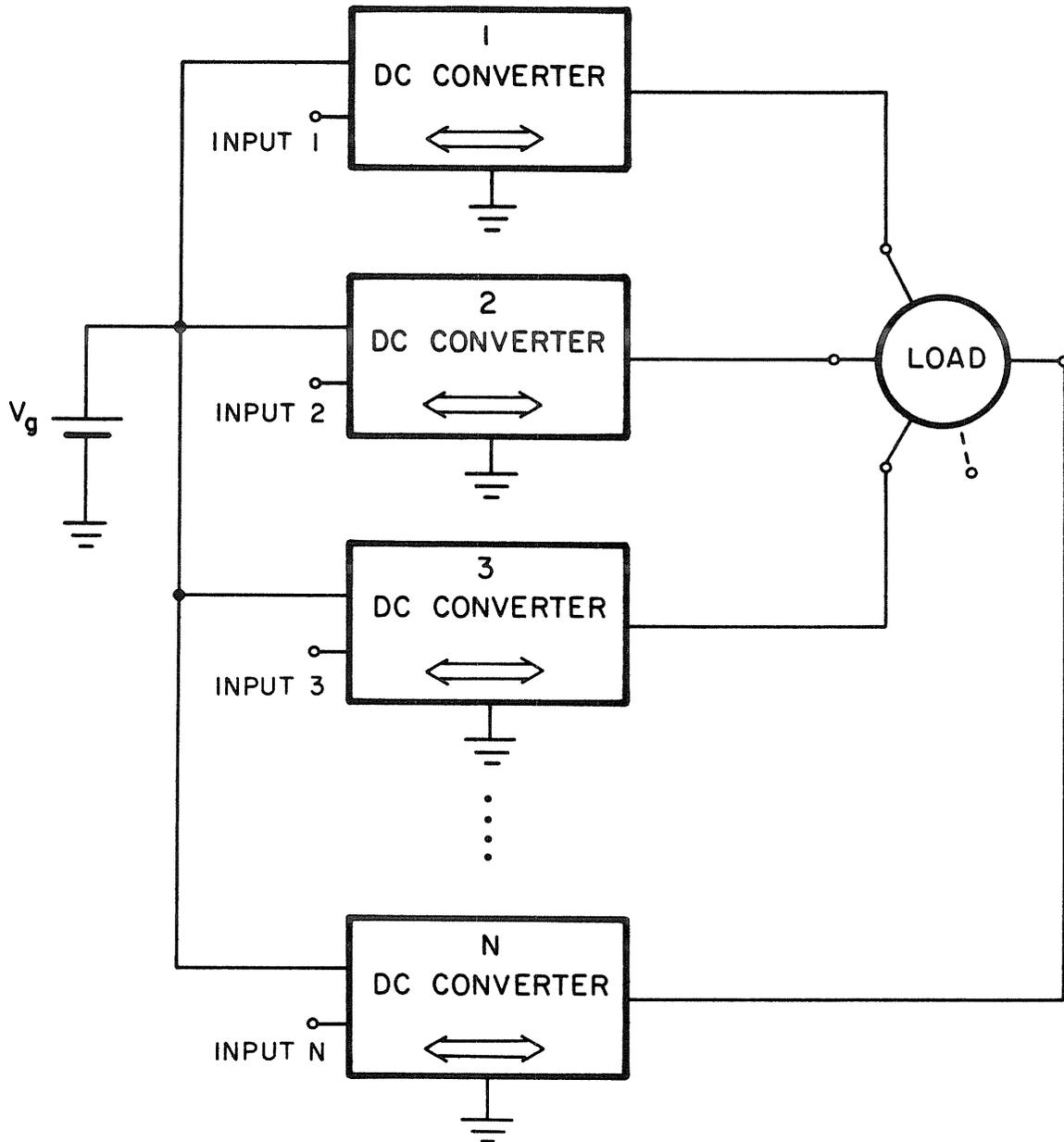
Fig. 12.7 Extension of three-phase converter of Fig. 12.4 to a general polyphase amplifier. Modulators are inclusive to the converters and a set of polyphase sine waves drives the inputs.
