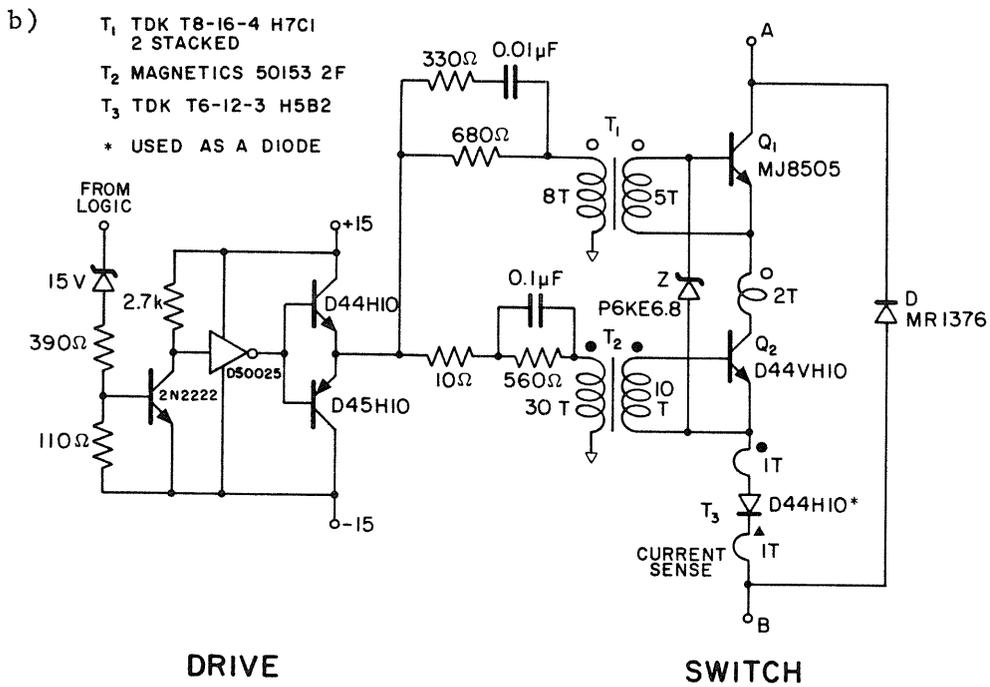
Fig. 13.1 (a) Buck three-phase variable speed motor drive. (b) Practical implementation of one switch and its drive.
