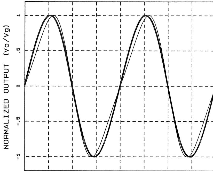
Fig. 12.8 Production of sine wave with gain of 1. Thick lines:  $D = 0.8$ ,  $a = 0.0228$ . Thin lines:  $D = 0.3$ ,  $a = 0.243$ .
