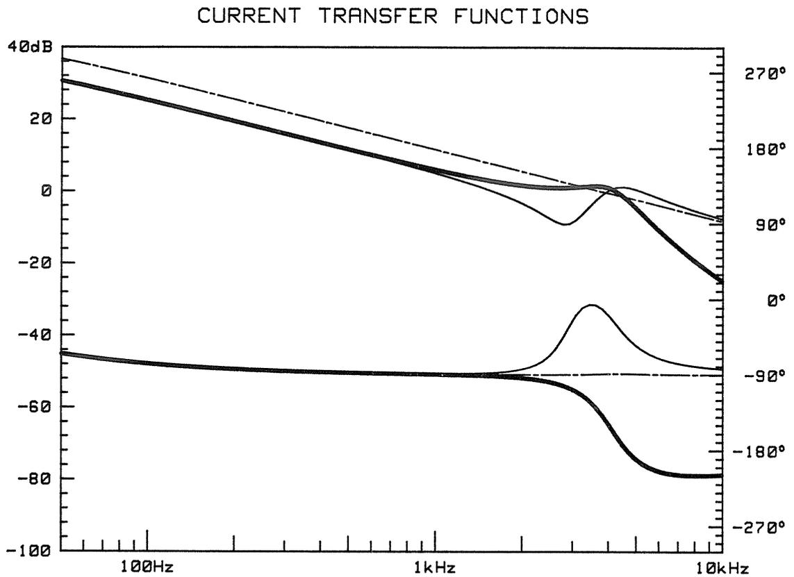
Fig. 8.6 Current transfer functions of the Ćuk battery charger. Thick lines are for  $\hat{i}_2/\hat{d}$ , thin lines are for  $\hat{i}_1/\hat{d}$ , and dash-dot lines are for  $(\hat{i}_1 + \hat{i}_2)/\hat{d}$ .
