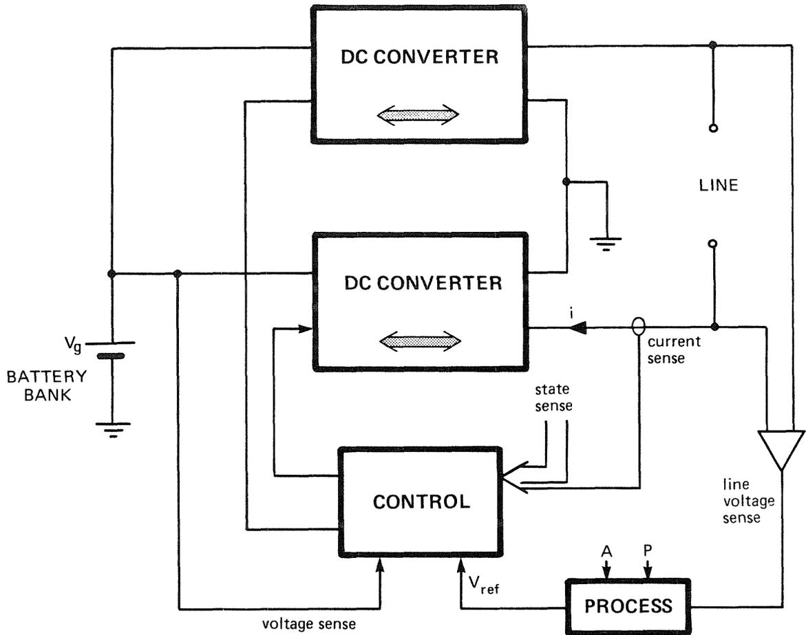
Fig. 8.1 Basic structure of the battery charger. The control circuit causes current to be proportional to the reference signal which itself is an amplitude-phase adjusted replica of the input voltage.
