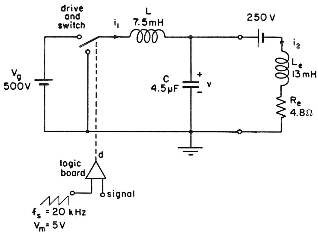
Fig. 13.6 Open-loop model of one stage with the other stages regulated.
