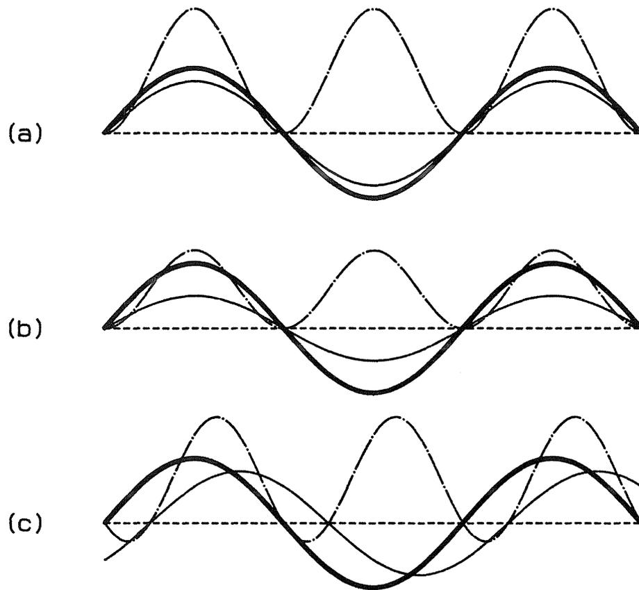
Fig. 8.2 Modes of operation of the battery charger. (a) High power resistive, (b) low power resistive, and (c) inductive. The voltages, currents, and powers are represented by thick, thin, and dash-dot lines, respectively.
