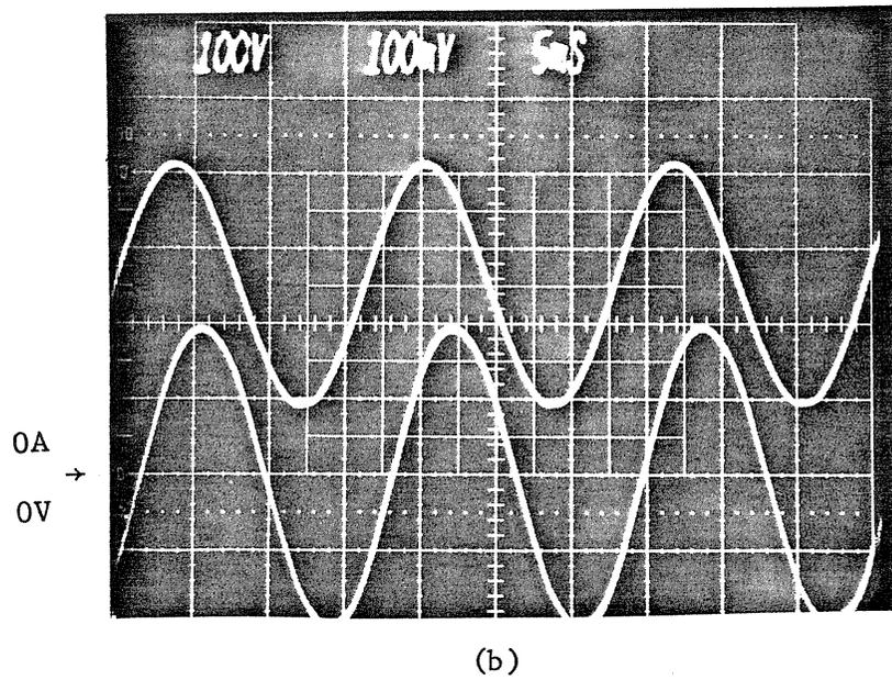
Fig. 13.11 Current and line-to-ground voltage waveforms of the motor drive, (a) output at 20 Hz with no load. (b) 60 Hz operation with more than 0.8 hp mechanical load. Current scales: 2A/div.
