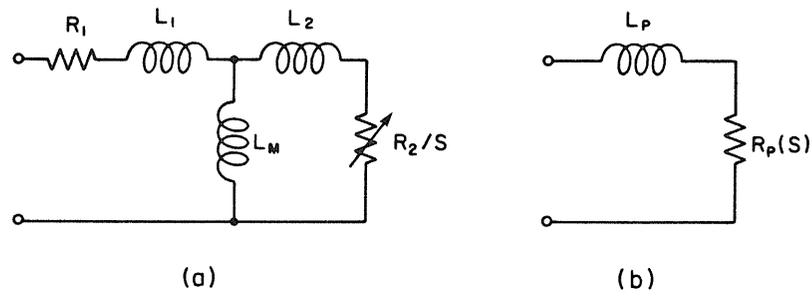
Fig. 13.4 (a) Steady-state model for one phase of an inductor motor. (b) Simplified version for modelling purposes.
