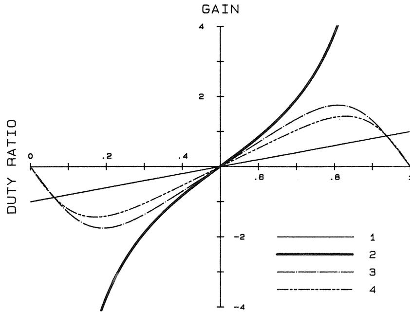
Fig. 7.4 Dc gain characteristics of various push-pull amplifiers. (1) Ideal buck, (2) ideal others, (3) linearized Ćuk, and (4) linearized boost and buck-boost.
