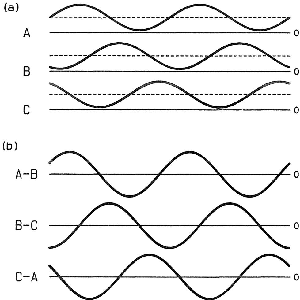
Fig. 12.5 (a) Line-to-ground and (b) line-to-line voltages generated by the new three phase power amplifier. The dc component of the line-to-ground voltages automatically disappears in line-to-line voltages which are pure ac.
