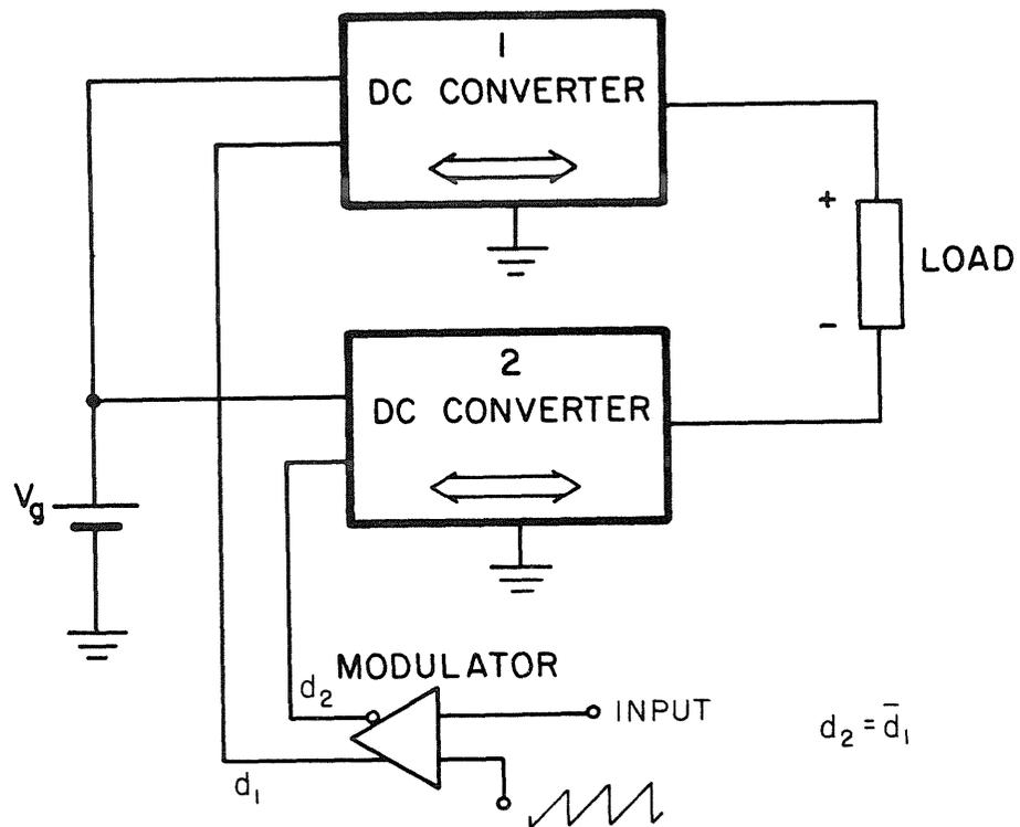
Fig. 6.9 A general push-pull switching power amplifier. Arrows denote current-bidirectionality.
