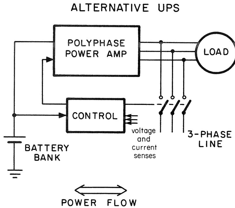
Fig. 14.3 Alternative three-phase UPS comprising only one polyphase power amplifier.
