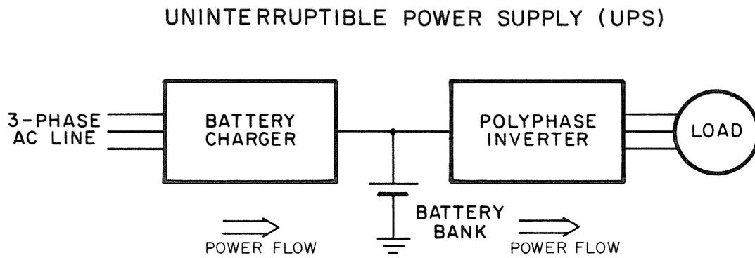
Fig. 14.1 A three-phase uninterruptible power supply utilizing a polyphase amplifier.
