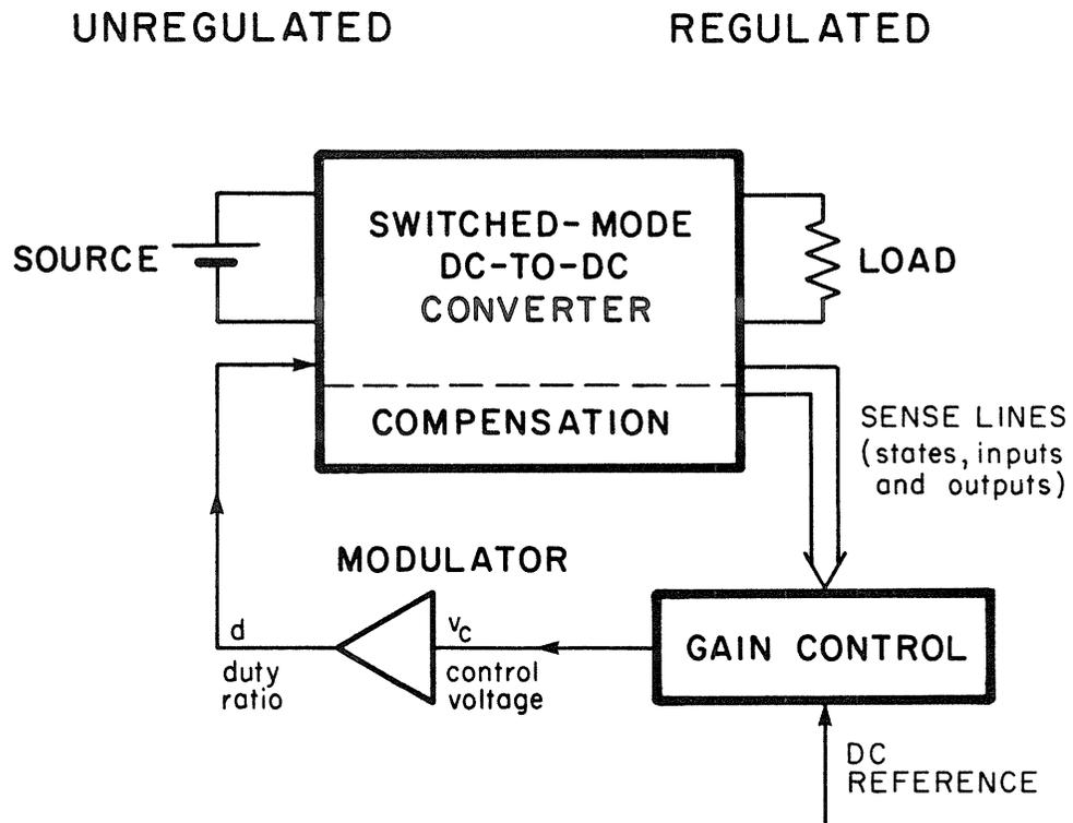
Fig. 1.2 Switching regulator: Full-state feedback regulation of the output.
