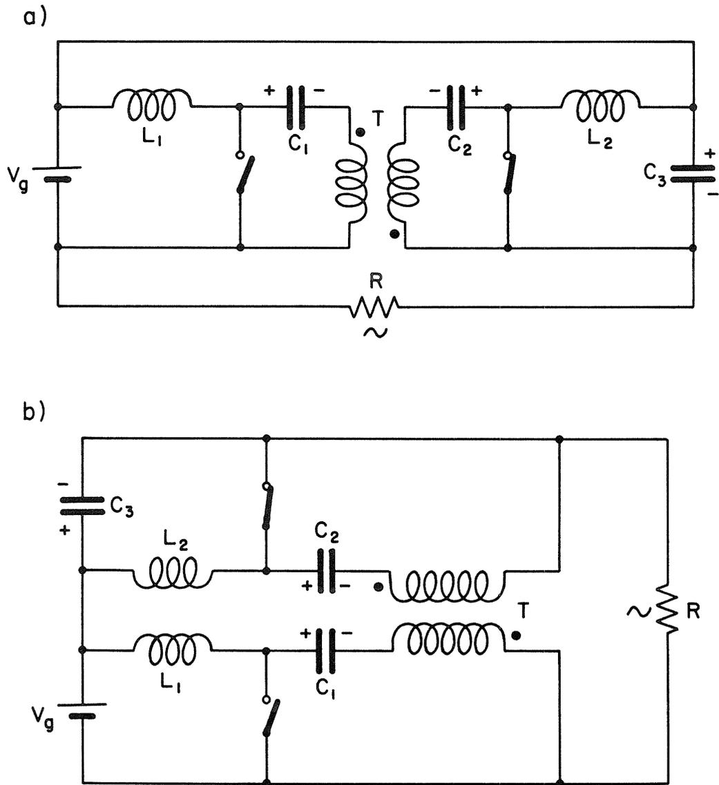
Fig. 6.7 Differential ac generation by use of a Cuk converter. (a), (b) same amplifier drawn differently.
