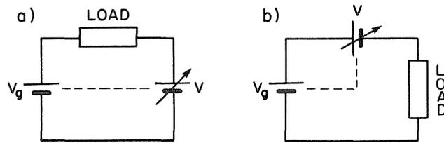
Fig. 6.5 Differential generation of ac. (a) Floating load. (b) Output voltage is grounded on one side.
