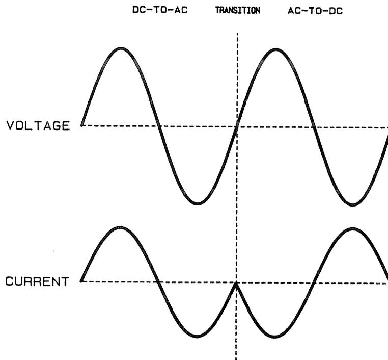
Fig. 9.2 Transition from the inverter mode to the charger mode.
