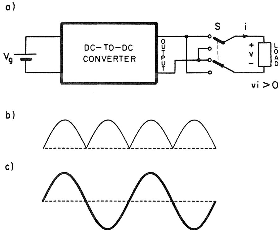
Fig. 6.4 Two-quadrant ac generation. (a) The basic method. The switches reverse the polarity of voltage. (b) Output voltage of the dc converter. (c) The load voltage.
