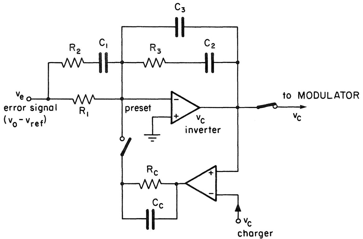
Fig. 9.5 Voltage preset circuit for the inverter control circuit.
