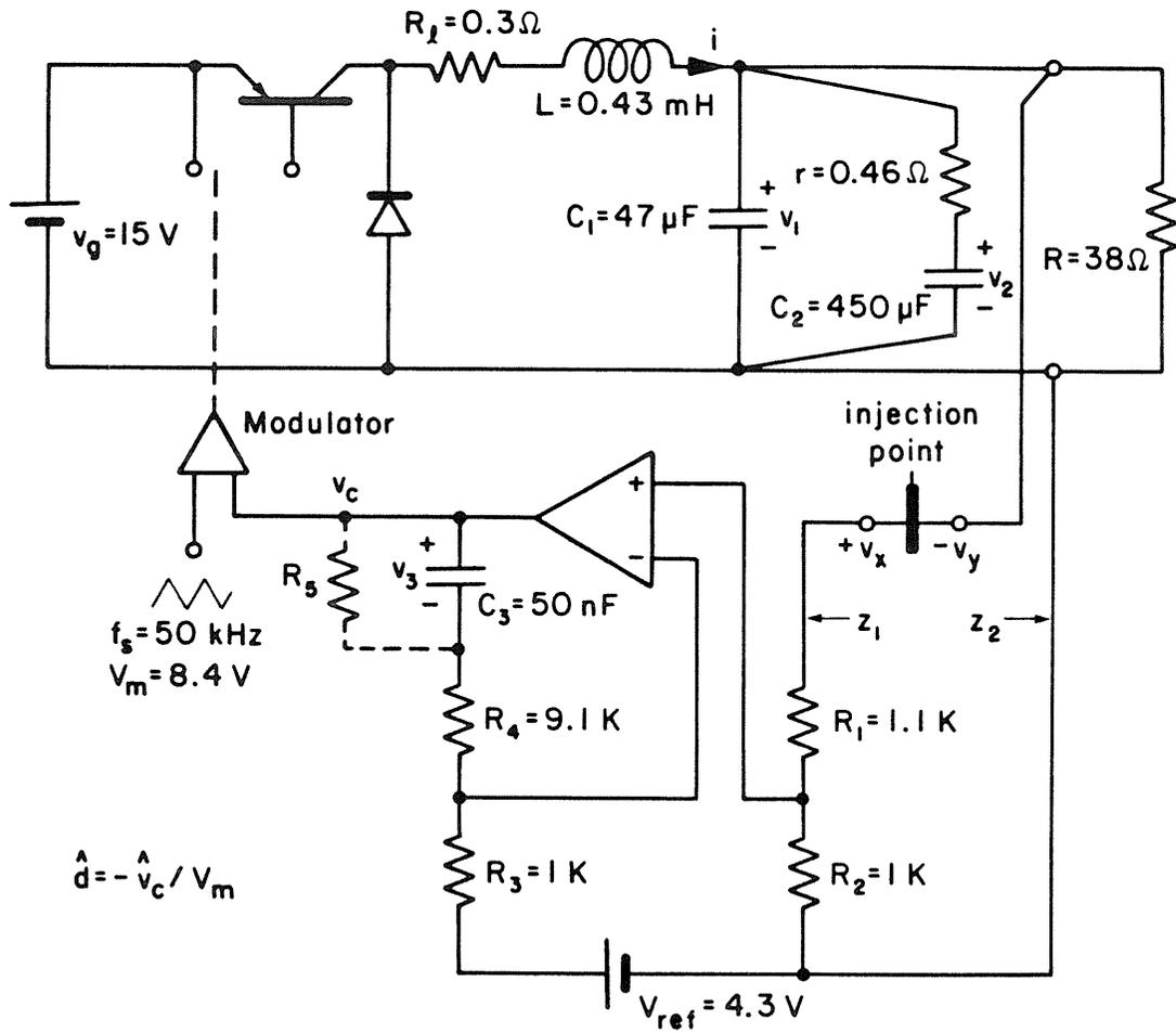
Fig. 3.4 Closed-loop buck example.
