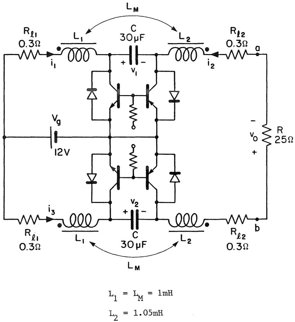
Fig. 7.8 Experiment coupled-inductor Ćuk amplifier.
