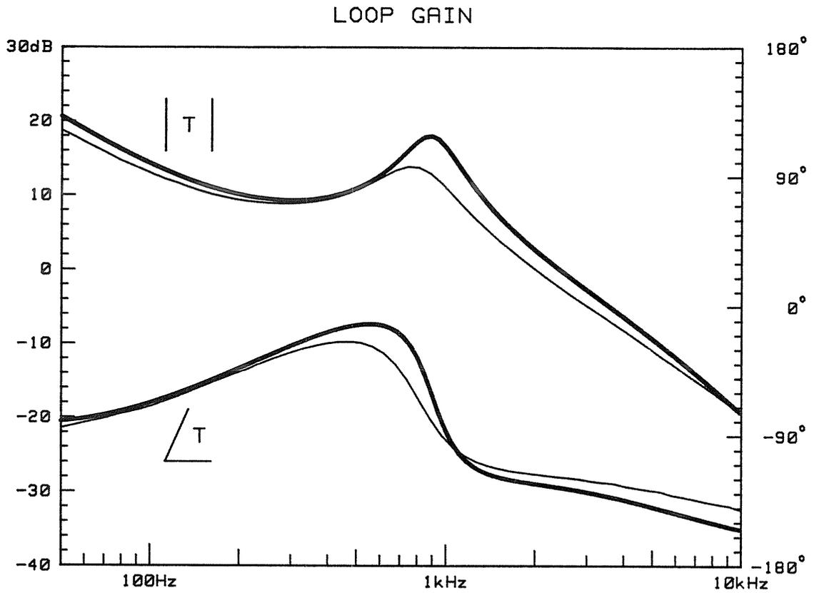
Fig. 13.8 Comparison of theoretical prediction (thick lines) and practical measurement (thin lines) of the loop gain of one converter.
