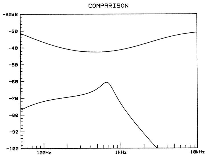
Fig. 13.10 Comparison of the two sides of Equation (13.13). Upper graph is the magnitude of  $H(s)$  and the lower one is for  $2/9\alpha^2A$ .
