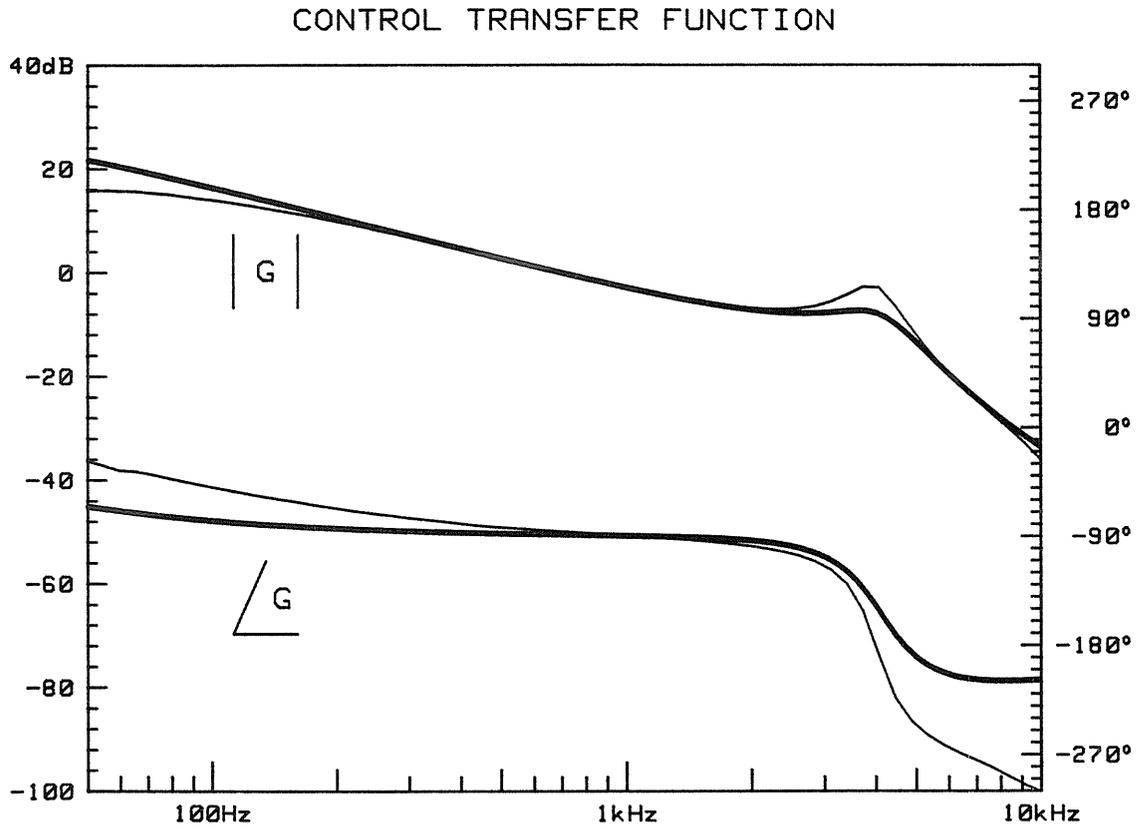
Fig. 8.5 Control-to-output current transfer function of the Ćuk battery charger. Thick and thin lines correspond to predicted and measured results.
