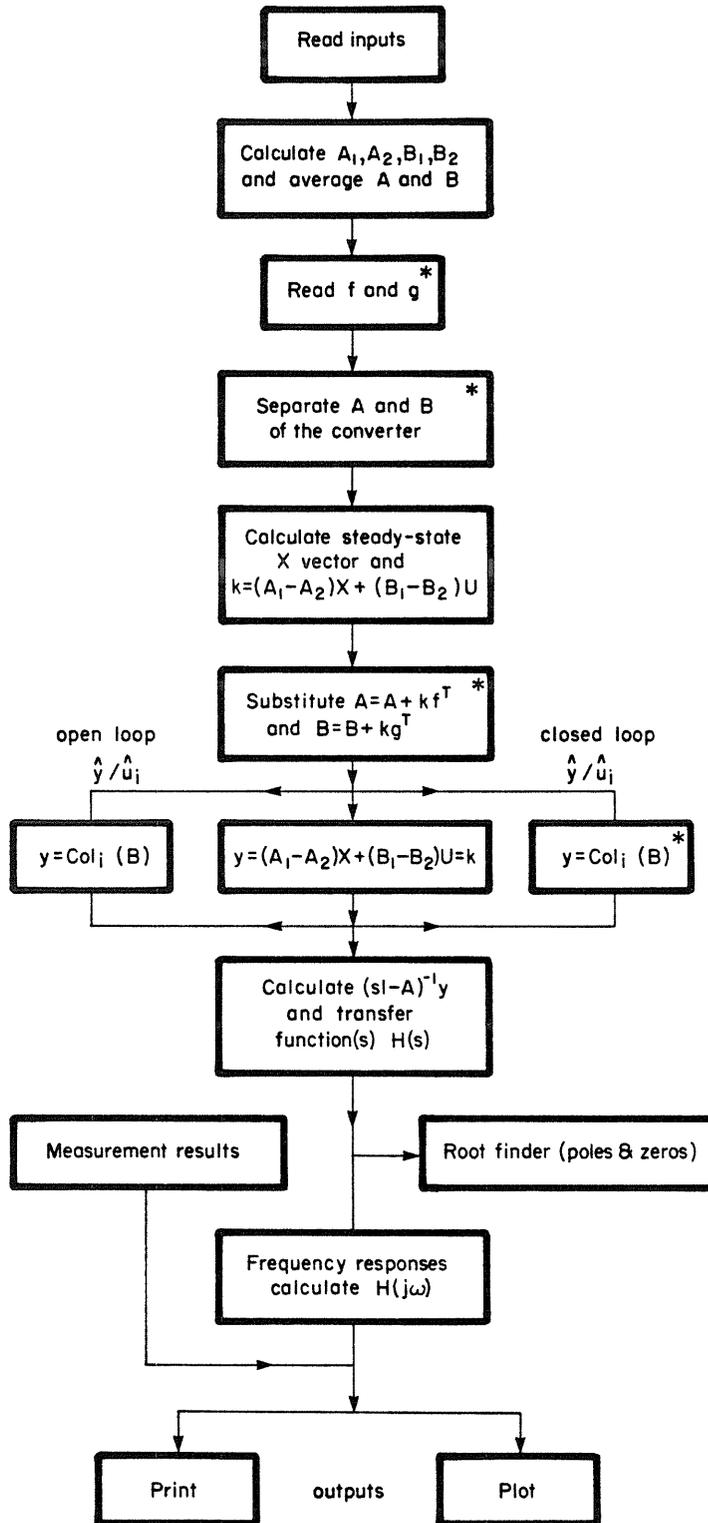
Fig. 3.2 Flowchart of Switching Converter Analysis Program (SCAP): blocks with asterisks are used in closed-loop calculations only.
