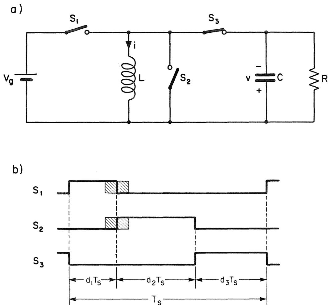
Fig. 7.6 (a) Linearized buck-boost converter (b) timing for the switches.
