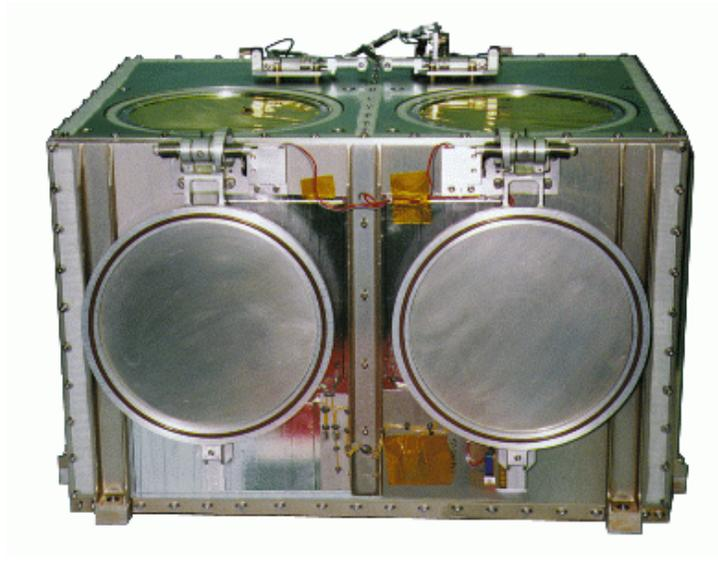
Figure 3.6: The SIS instrument. There are two detector stacks in the instrument. The two large roundels are covers that were opened after launch. From Stone *et al.* (1998a).
