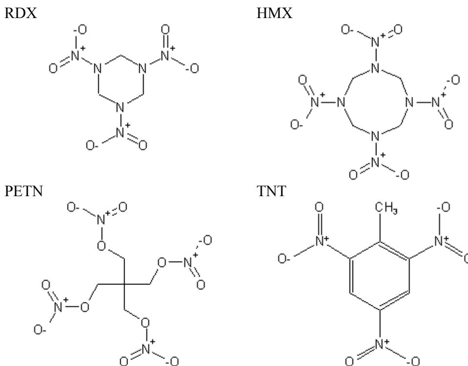
**Figure 2.1** Molecular structure of the four military grade explosives examined.
