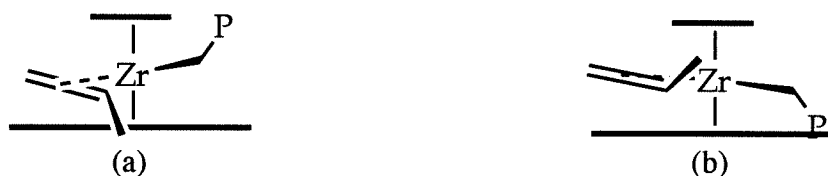
Figure 7. Monomer-Polymer Conformation with Achiral \beta -Carbon (a) re Face (b) si Face
