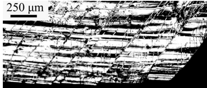
Figure 3.4 – Side view of a bending sample of \text{Cu}_{47.5}\text{Zr}_{47.5}\text{Al}_5 showing shear band offsets and shear band spacing. The sample was unpolished on the sides so horizontal lines are flow lines from casting, not from deformation. When the shear band offset become too large (at some specific shear band length) cracks nucleate and the beam fractures.
