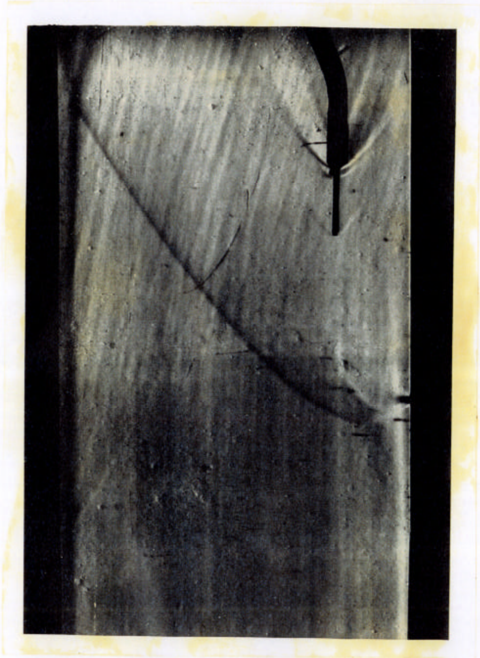
Fig. 7. Schlieren Picture of Flow Field with Three-Dimensional Injection and a Laminar Boundary Layer. M_{\infty} = 2.610 , P_0/p_0 = 30.2 .
