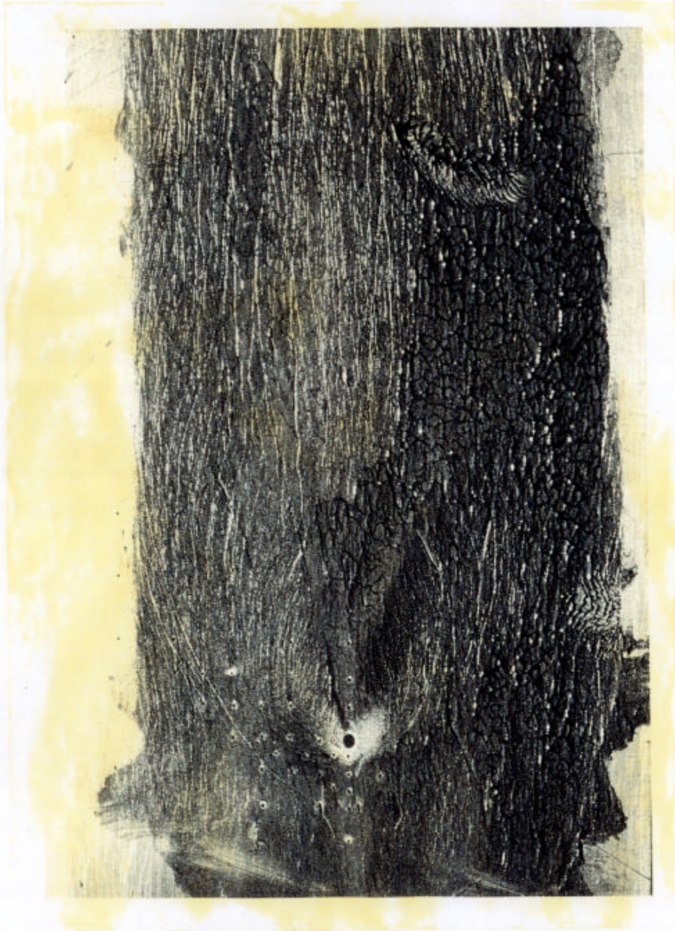
Fig. 21. Photograph of Injector Plate Showing Effect of Boundary Layer Flow upon Grease Mixture During Three-Dimensional Injection at P_0/P_0 = 7.77 and a Turbulent Boundary Layer. M_\infty = 2.610 .
