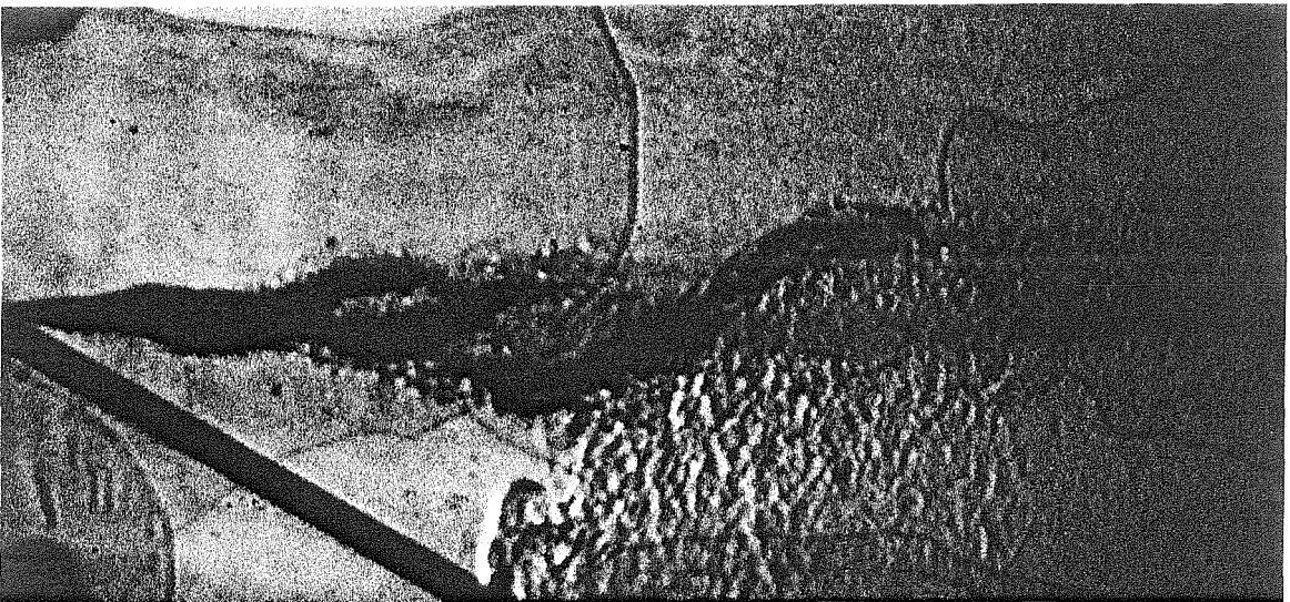
Fig. 4.4: Schlieren visualization after expansion turn; U_1 \cong 57 m/s [N 2 ] and U_2 \cong 6 m/s [He/Ar].
