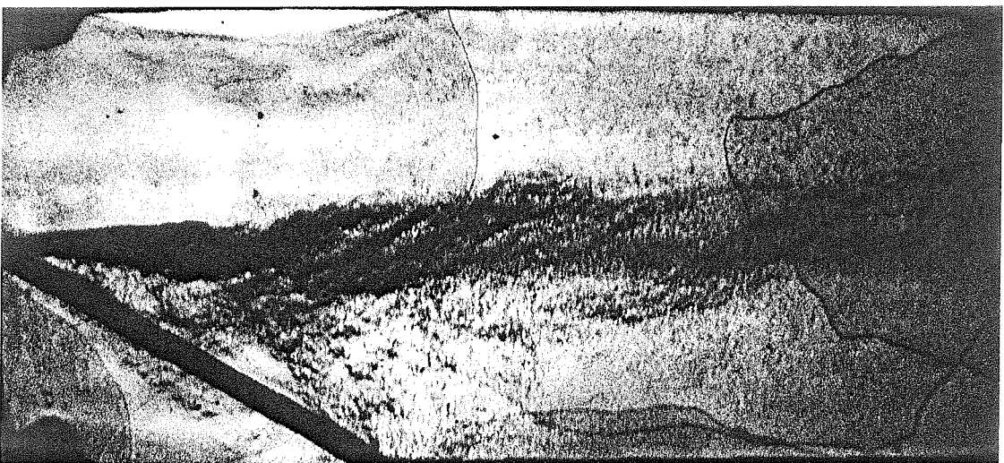
Fig. 4.12: Schlieren visualization after expansion turn; U_1 \cong 92 m/s [ N_2 ] and U_2 \cong 3 m/s [He/Ar].
