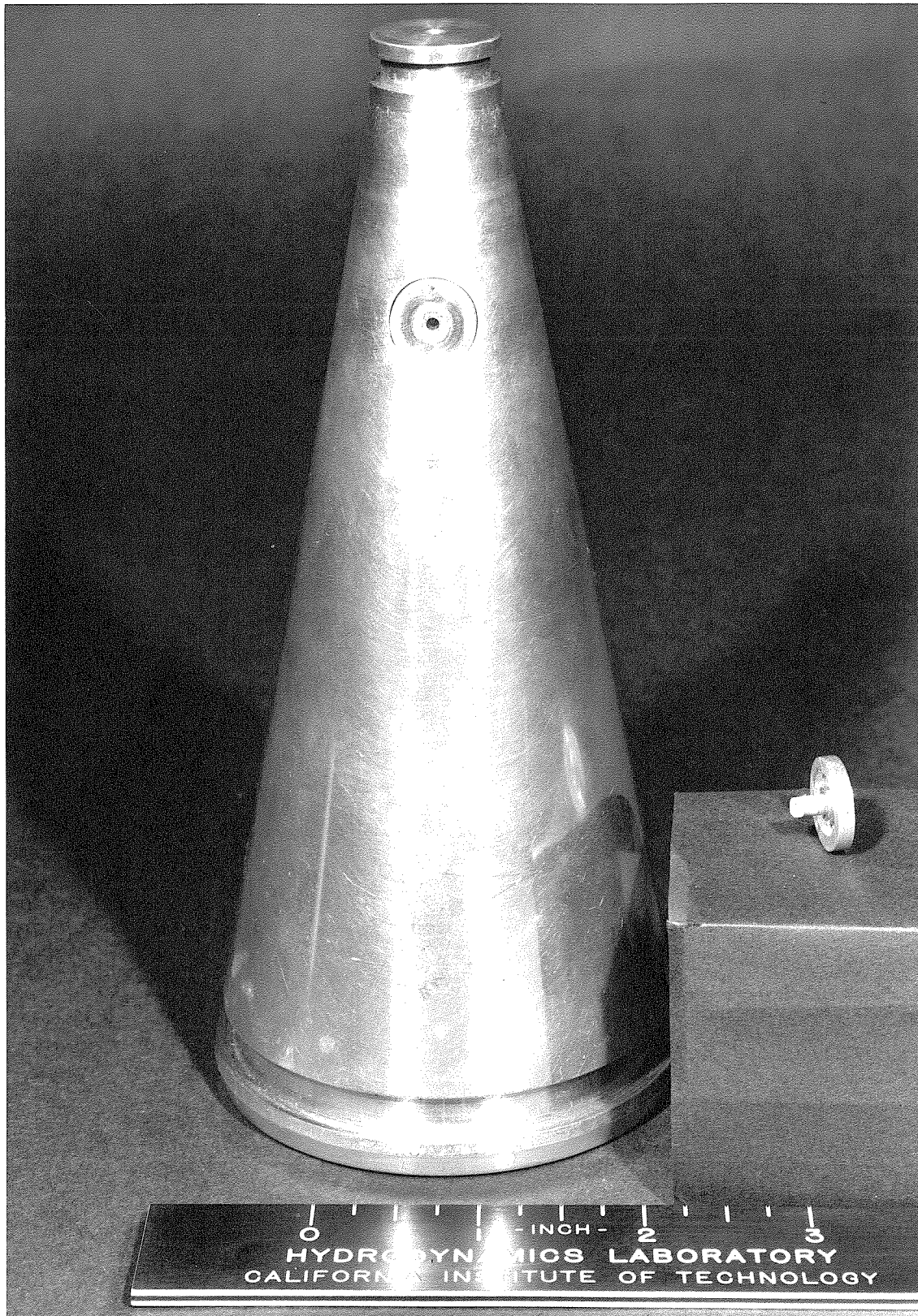
Fig. 22 Second Section of 10^\circ Half-Angle Cone with Windows
