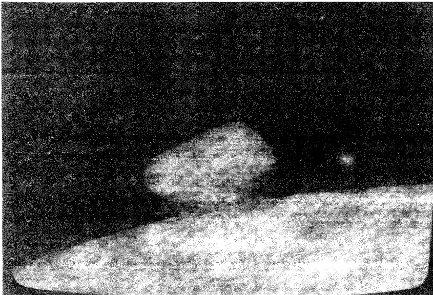
Fig. 4-24. A hologram of travelling bubble cavitation on the hemispherical body. Re_D = 3.8 \times 10^5 , \sigma = 0.63 . The photograph covers the region between x/D = 0.32 and x/D = 0.46 .
