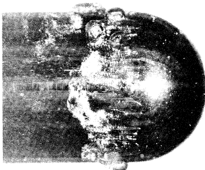
Fig. 4.18. A mixture of band and travelling bubble cavitation in a tunnel filled with a large number of bubbles. Re_D = 3.70 \times 10^5 , \sigma = 0.54 .
