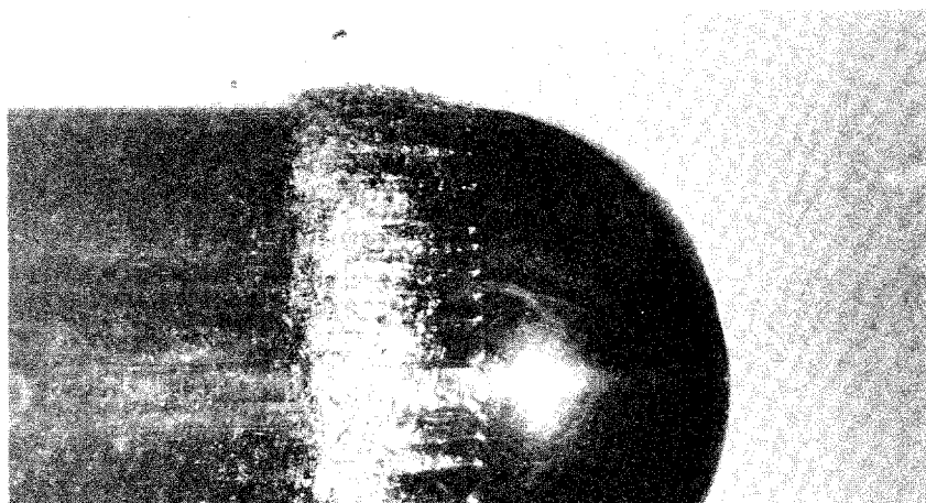
Fig. 4.17) Band type cavitation on the hemispherical body. Re_D = 3.70 \times 10^5 , \sigma = 0.55 .
