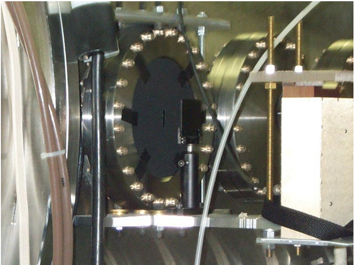
Figure 3.9. Opaque mask to prevent extraneous light from reaching the photomultiplier.
