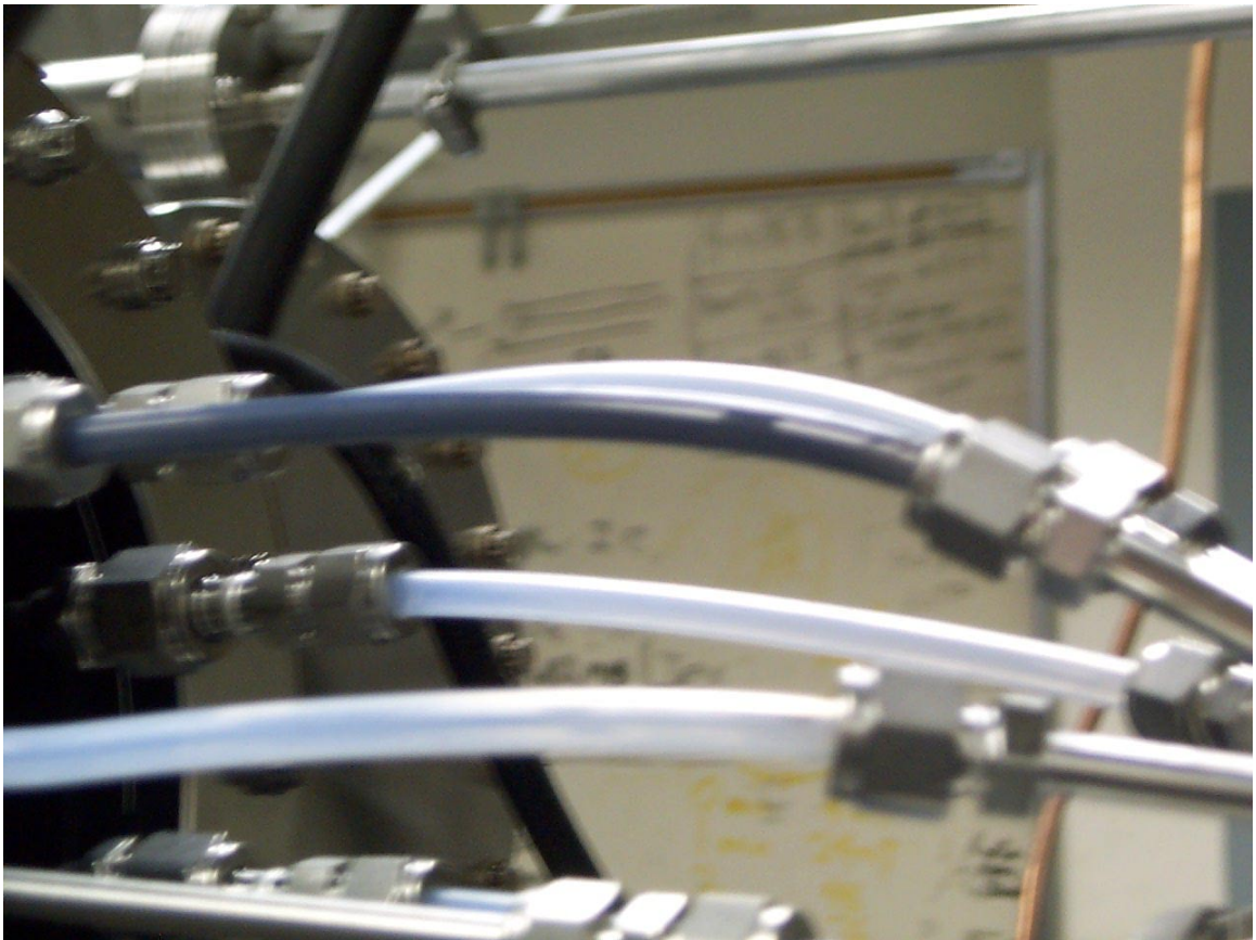
Figure 4.7. Gas injection line to the inner electrode after plasma breakdown has occurred in the Teflon tube, leaving a dark residue. A second power supply for the gas valve system has been added to the experiment to eliminate this problem.
