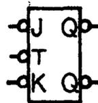
where transition is caused by T going from 1 to 0. In addition a reset lead is available forcing the Q output to a value of 0. The labeling system used by the manufacturer is shown in figure A15 however, the system in figure A14 is used extensively in the diagrams in this appendix because it seems strange to have an output labeled 1 whose value may be 0 or 1.
