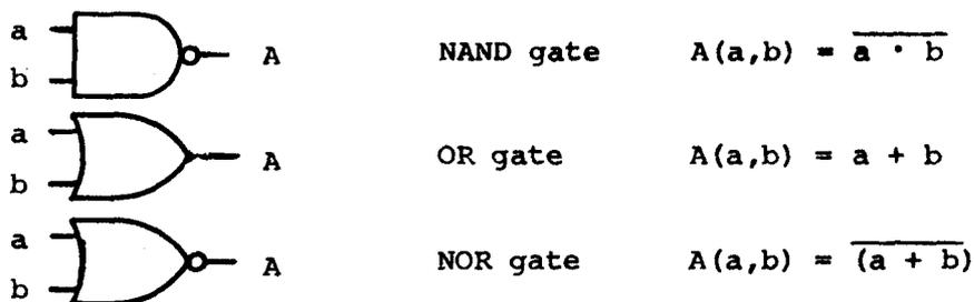
A small circle on an input or output of a symbol means that the input or output is inverted from what it would have been. The most common circuit element used in the Film Copier is a n-input NOR gate which is implemented electronically as shown in figure A 11. The inverter can be considered as a one input NOR gate and is implemented that way electronically.
