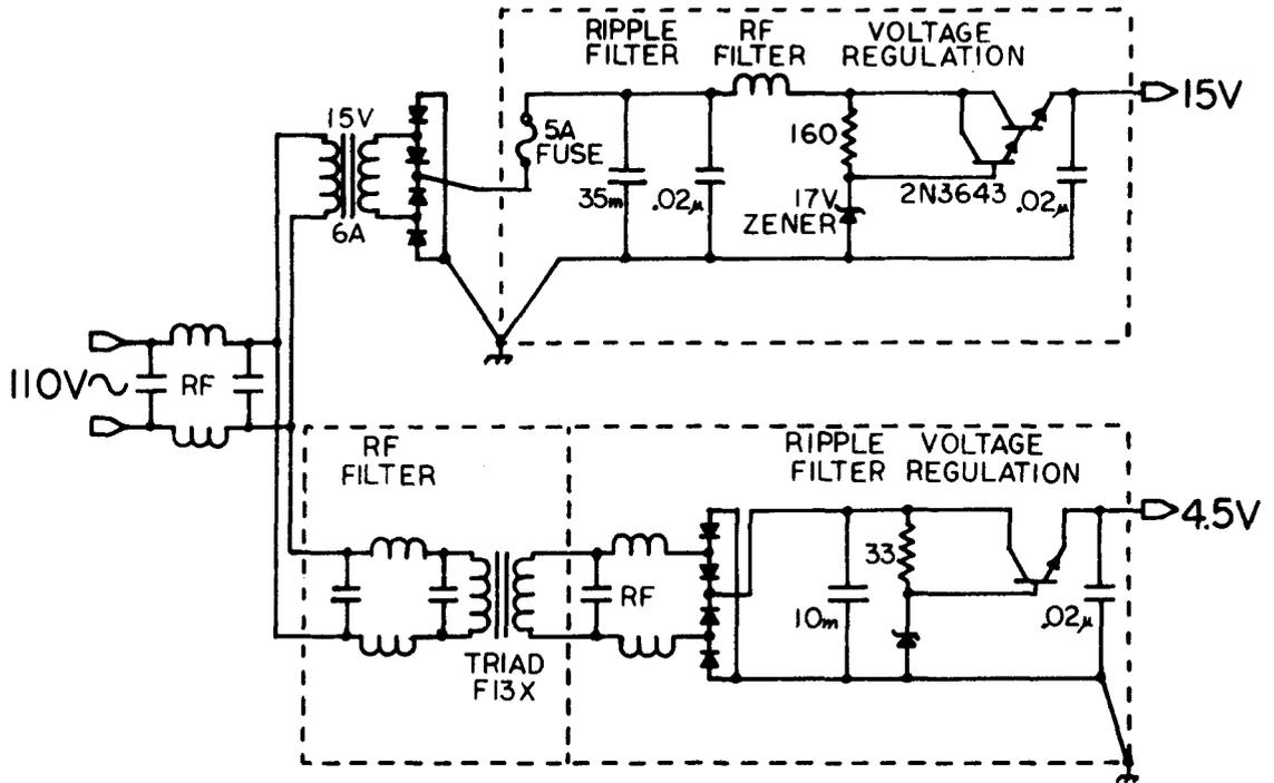
Figure A29 Optical Printer Power Supply
