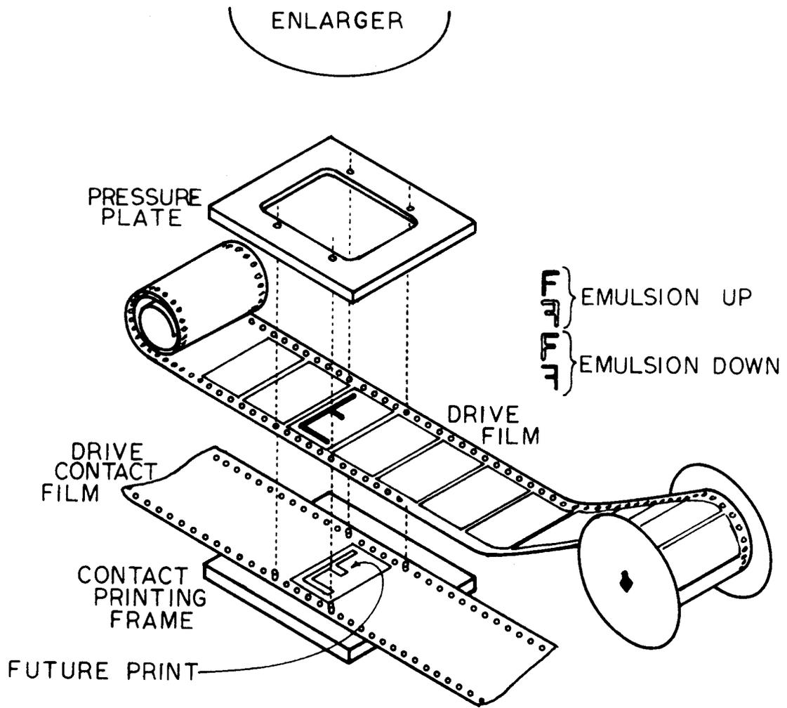
Figure A3 Step 1, Contact Printing Shown Schematically
