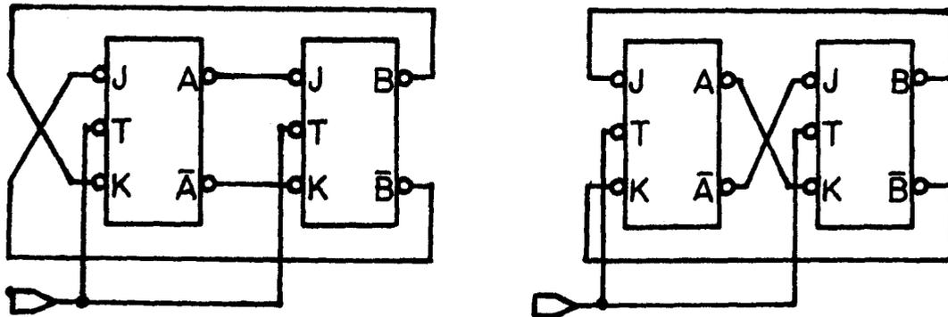
The 200 positions of the motor may be labeled each according to its electrical state; 0,1,2, or 3. The result is that position N has electrical state  $N \pmod{4}$ . There are 50 positions corresponding to each state. The motor always goes to the nearest position corresponding to a given state when states change. Clearly a change, from say state 0 to state 2 in a time small compared to the reaction time
