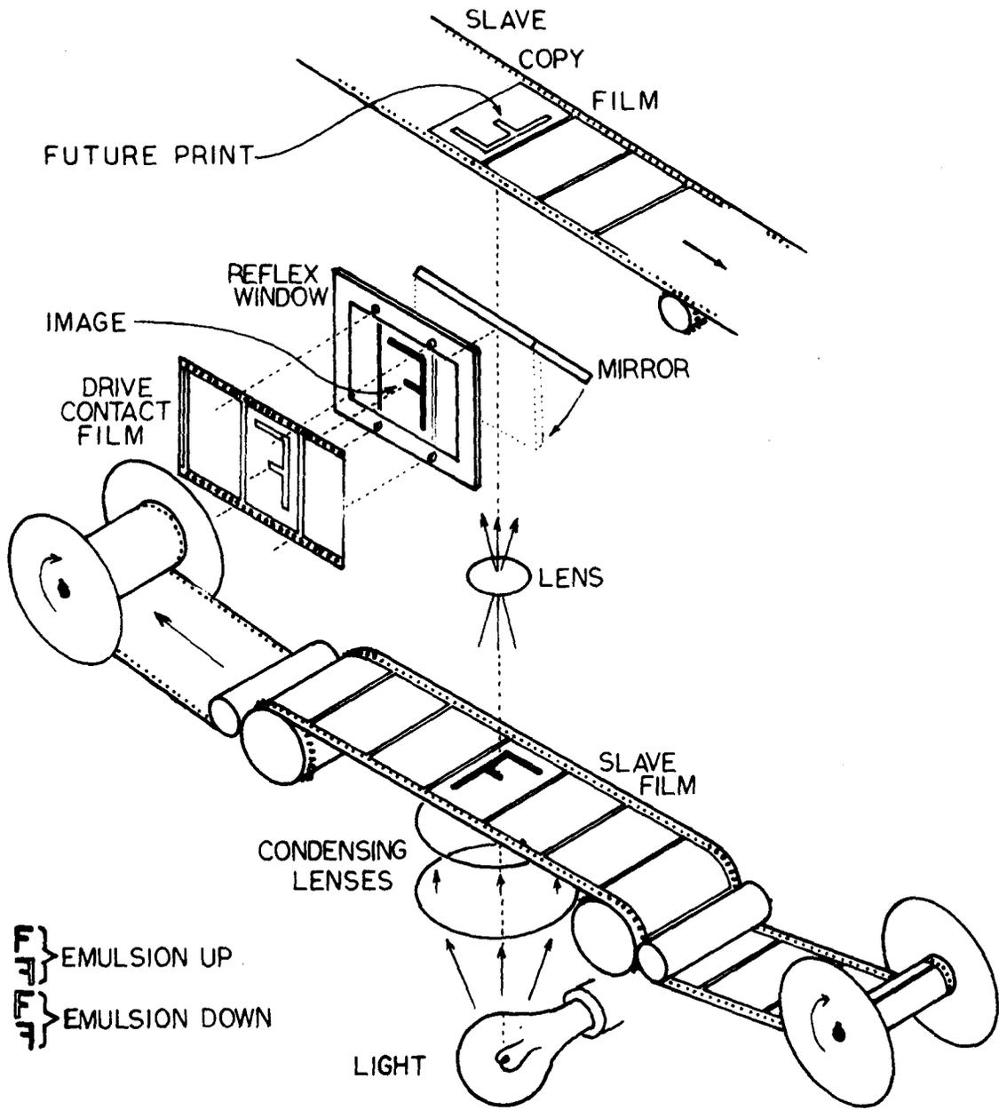
Figure A4 Step 2, Unit Magnification Alignment Copying
