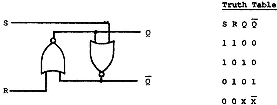
As shown in the truth table of figure A12 there are two stable states of the flip-flop when the inputs S and R are both 0. Either of these states may be attained by momentarily causing a 1 on either S or R. The state where both S and R are 1 is generally avoided, since it is usually desired that  $\bar{Q}$  have the opposite value of Q as its label implies. S-R flip-flops can be made from NOR gates having 3 or more inputs, thus providing extra independent S or R inputs.
