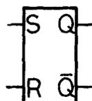
S and R are inputs and Q and  $\bar{Q}$  are outputs. An S-R flip-flop is usually constructed from two 2-input NOR gates as shown in figure
