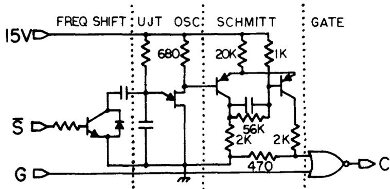
Figure A30 Optical Printer Clock
