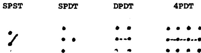
Push button switches, microswitches, relay contacts, and any other switch having normally closed and normally open contacts are symbolized as in figure A17 usually with contacts shown in normal position.
