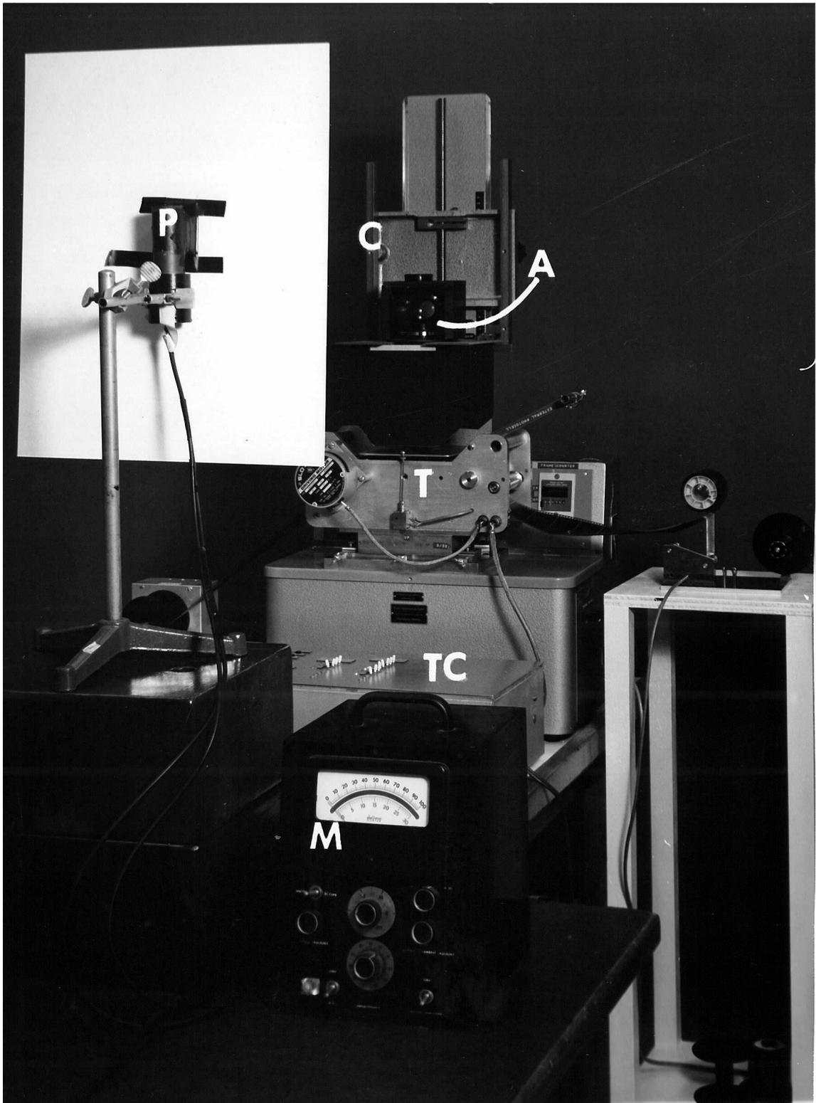
Figure 11. The Film Copier as a Microphotometer
