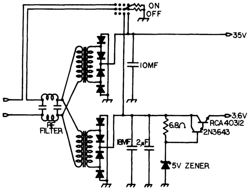
Figure A21 Transport Control Power Supply
