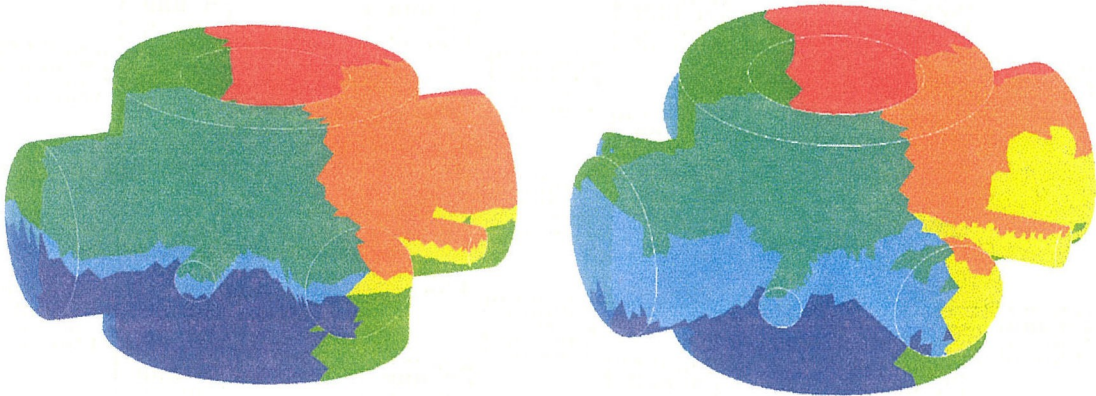
Figure 5.4: The grid for the GEC reference cell after initial partitioning (left) and static partition balancing (right)
