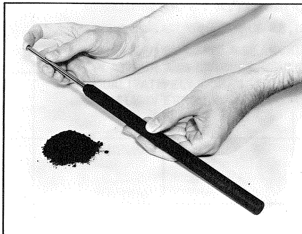
Fig. 5. METHOD FOR OBTAINING AN INTENSE IRON ARC FROM A CONVENTIONAL SEARCHLIGHT.
