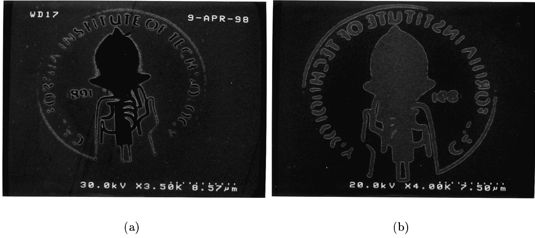
Figure 3.4: Projection results with B = 1.85T , V = 3kV : (a) mask; (b) sample.
