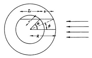
Let r be the radius of the ionization chamber, R-r the thickness of the shield, s the path length in the shield for a primary particle coming in the indicated direction, L its path length in the chamber and Q,ø the polar angles
