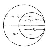
$$S(r) = S_{r_0-r}(0) + \pi \left[ r_0^2 - (r_0-r)^2 \right] \rho(r_0) \qquad \text{for } r \leq 3 \times 10^{-4}$$
