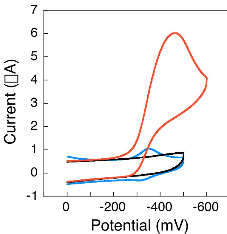
**Figure 2.4.** Cyclic voltammograms ( $\nu = 100 \text{ mV/s}$ ,  $A = 0.02 \text{ cm}^2$ ) of  $2.0 \text{ mM Fe(CN)}_6^{3-}$  plus  $2.0 \text{ }\mu\text{M MB}^+$  at a gold electrode modified with the thiol-terminated sequence SH-5'-AGTACAGTCATCGCG-3' hybridized to a fully basepaired complement (red) and a complement that features an A opposite the underlined C (black).
