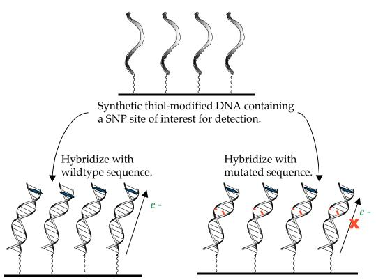
Fully matched duplex allows flow of current to the intercalator.
