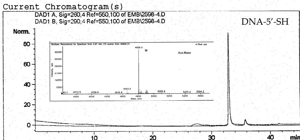
**Figure A.4.** Ellman's test for the detection of free thiols via HPLC analysis.
