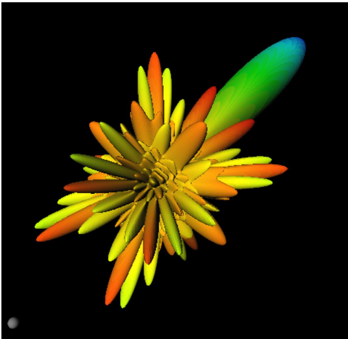
Figure 5.12: Far Field Intensity ( $|u_\infty|^2$ ) for Array of Smooth Scatterers –  $5\lambda \times 5\lambda \times 5\lambda$
