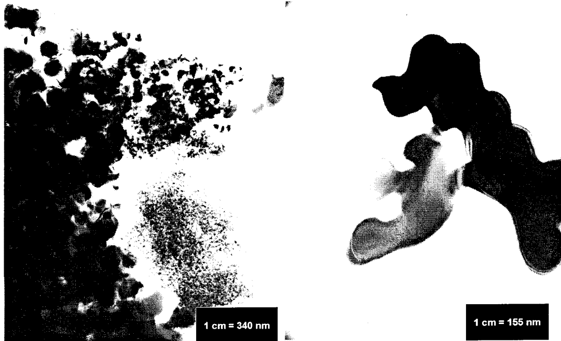
Figure 2.11: TEM micrographs of Linde A Al 2 O 3 particles showing trimodal distribution (left) and "limbs" (right).
