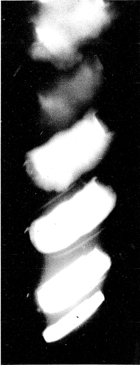
Fig. 28. Kerr cell photograph of 1.0 mil diameter aluminum wire in air
