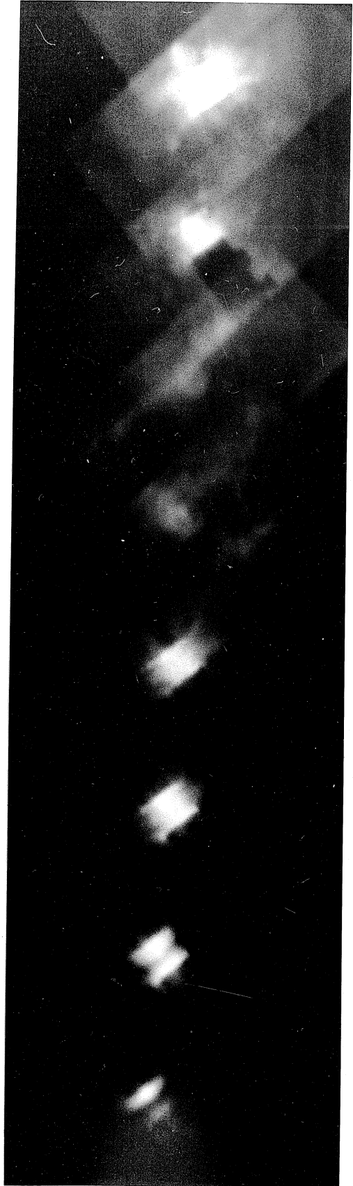
Fig. 44. Kerr cell photograph of 3.0 mil diameter iron wire in vacuum
