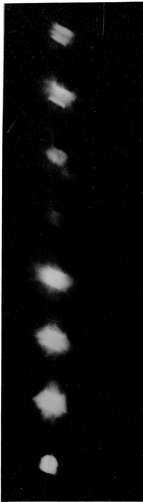
Fig. 49. Kerr cell photograph of 2.0 mil diameter copper wire in vacuum
