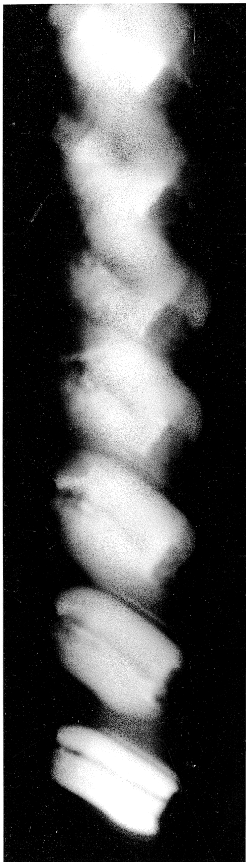
Fig. 22. Kerr cell photograph of 1.0 mil diameter silver wire in air
