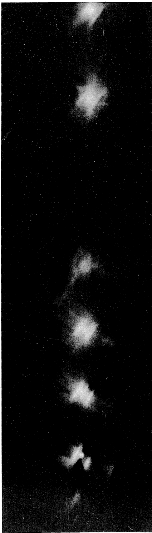
Fig. 51. Kerr cell photograph of 2.0 mil diameter tungsten wire in vacuum
