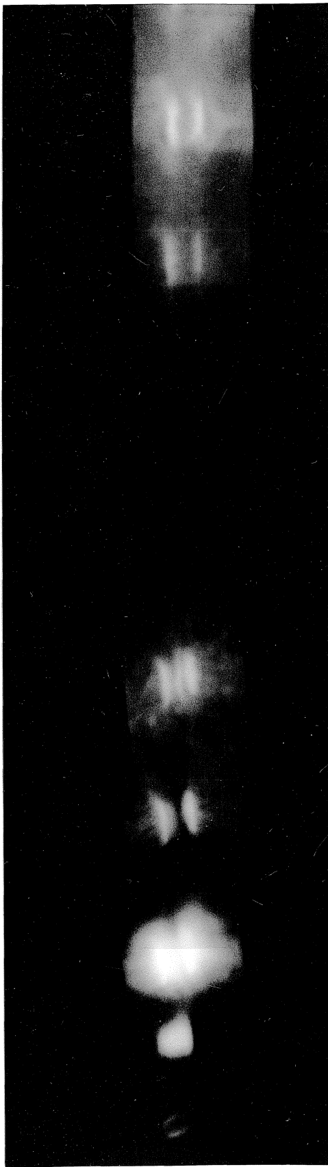
Fig. 50. Kerr cell photograph of 1.0 mil diameter copper wire in vacuum
