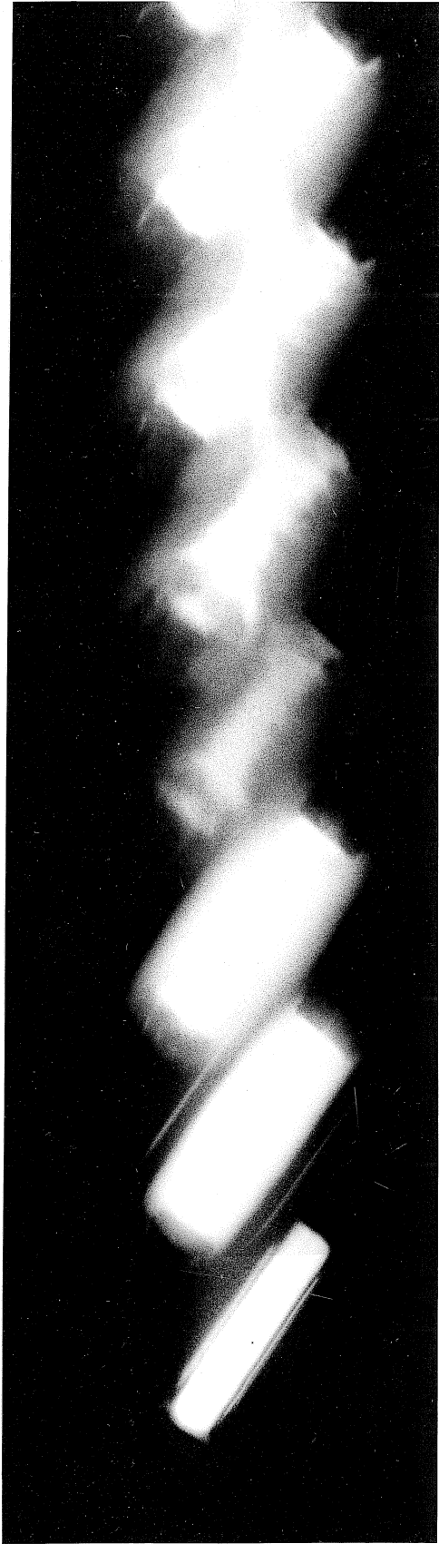
Fig. 27. Kerr cell photograph of 0.5 mil diameter tungsten wire in air
