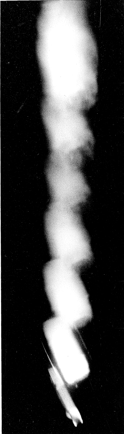
Fig. 24. Kerr cell photograph of 2.0 mil diameter copper wire in air
