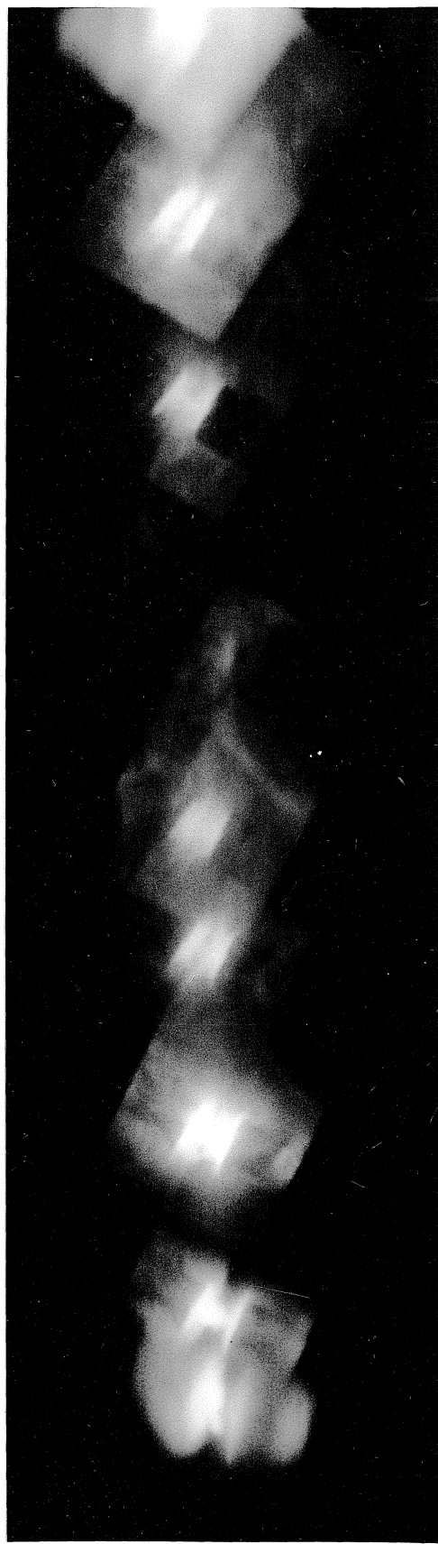
Fig. 52. Kerr cell photograph of .5 mil diameter tungsten wire in vacuum
