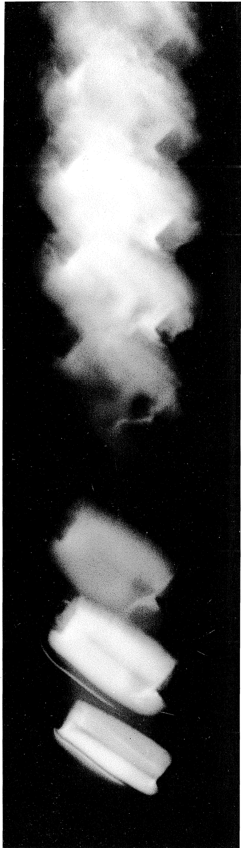
Fig. 21. Kerr cell photograph of 2.0 mil diameter silver wire in air
