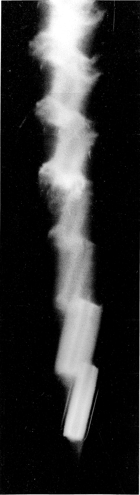
Fig. 26. Kerr cell photograph of 2.0 mil diameter tungsten wire in air
