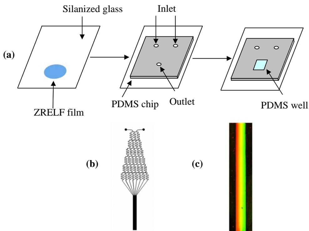
**Scheme 3.1** The assembly of microfluidic device and gradient generation. (a) Steps to assemble the setup to generate gradients. (b) Schematic design of the gradient generator. (c) Fluorescent image of the counter-gradient of QKZE and FNZE across the output channel.
