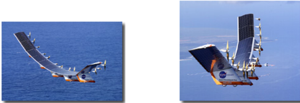
Figure 1.1: Helios Prototype long duration solar powered flight (courtesy NASA Dryden Flight Test Center).
