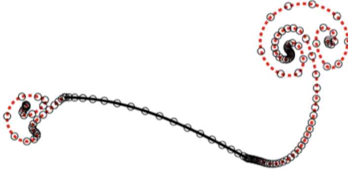
Figure 4.2: A diagram of the bound vortex sheet (black solid line) on a moving flexible plate and the generated free vortex sheet (red dash line). The bound and free vortex sheets are discretized into vortex filaments (circles).
