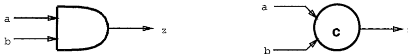
FIGURE 2.1. Schematic representation of AND gate and C-element A two-input AND gate with inputs a and b and output z has production rules:
