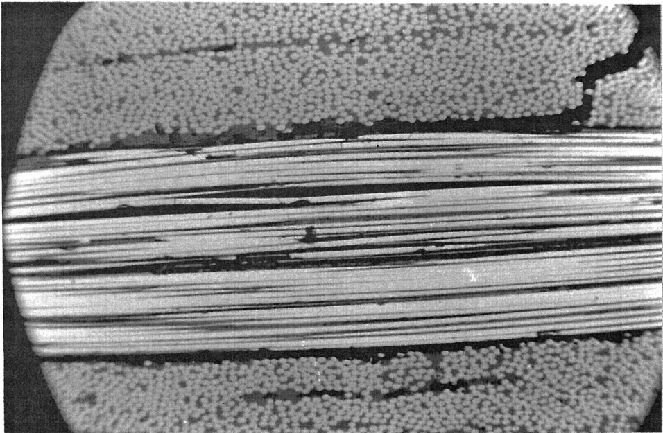
Figure 12g. Close-up of the region near the left of Figure 12f, where 45/0 delamination began.
