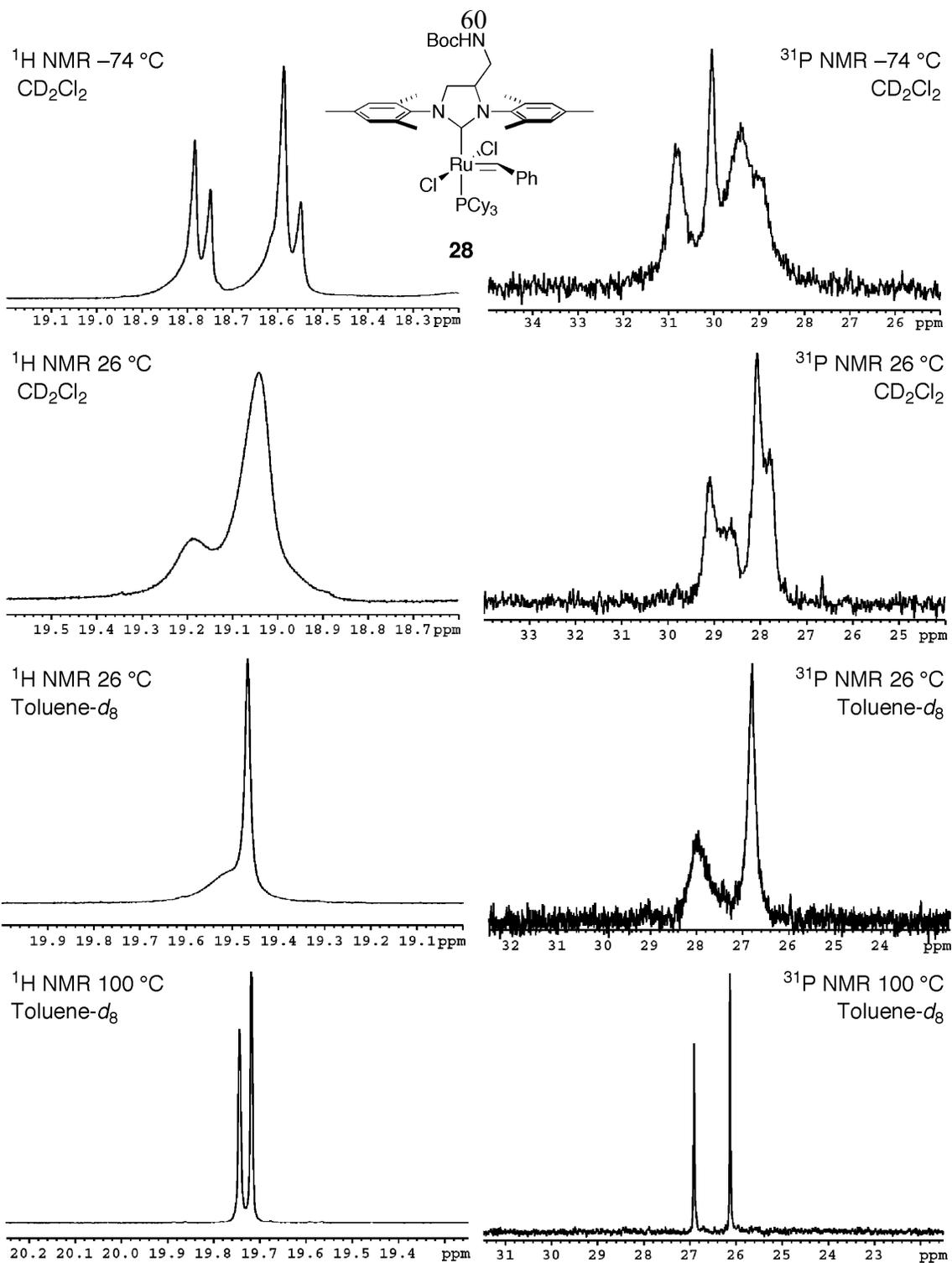
**Figure 3.2.** The NMR spectra of ruthenium complex **28** show fully reversible, temperature-dependent behavior. For clarity, only the benzylidene proton resonances of the  $^1\text{H}$  NMR spectra are shown.
