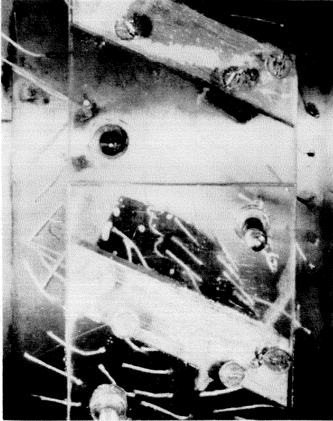
h. Downstream of Rotor (or Stator Inlet; Blades Shown are Stators); CS; R_T = 2010 ; \phi = 0.285
