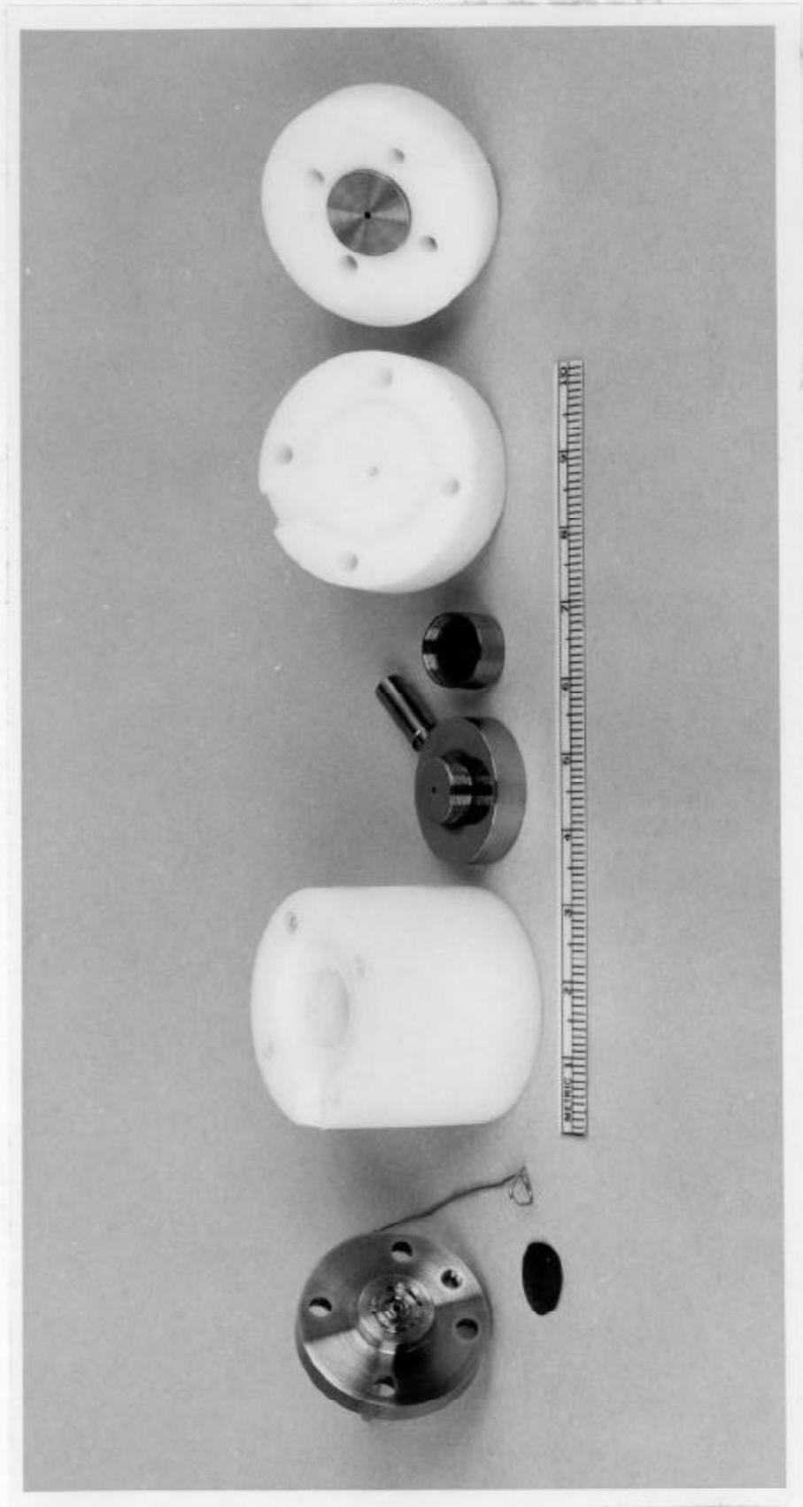
Figure 6. Exploded view of Plane-Parallel Detector.
