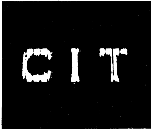
Figure 3.12 : High contrast image obtained from disk using diffractive readout scheme of Figure 3.11a.
