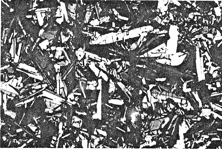
Plate 1a. Photomicrograph of section 68415.8 (crossed polarizers) illustrating typical intersertal texture. Field of view 2.1 \times 3.2 mm.
