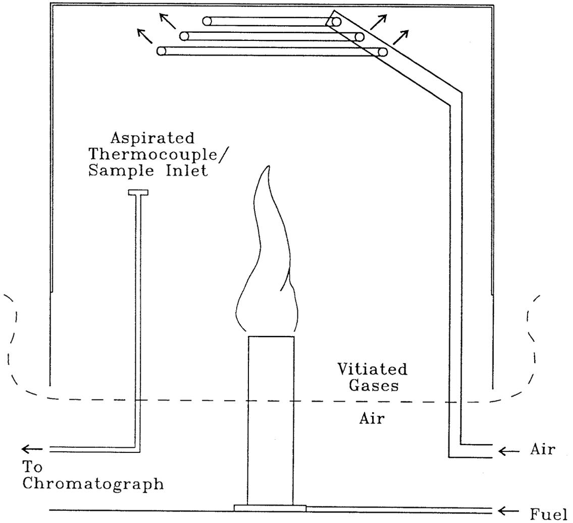
Figure 7.1: Schematic of experiment showing extending curtain which prevents entrainment
