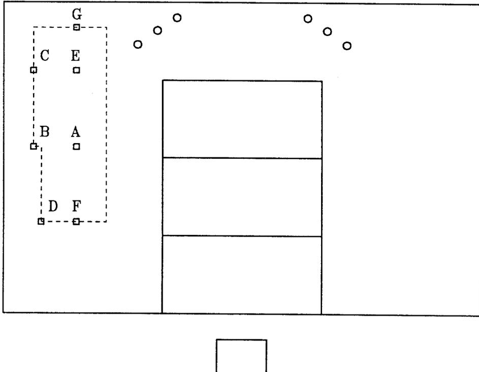
Figure 3.1: Range of possible probe positions with an interface height of 10 cm
