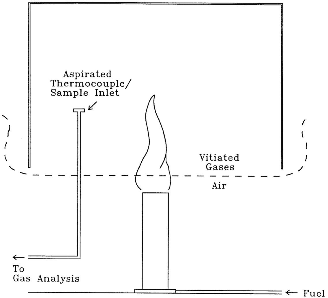
Figure 2.1: Schematic of experimental apparatus used in previous investigations
