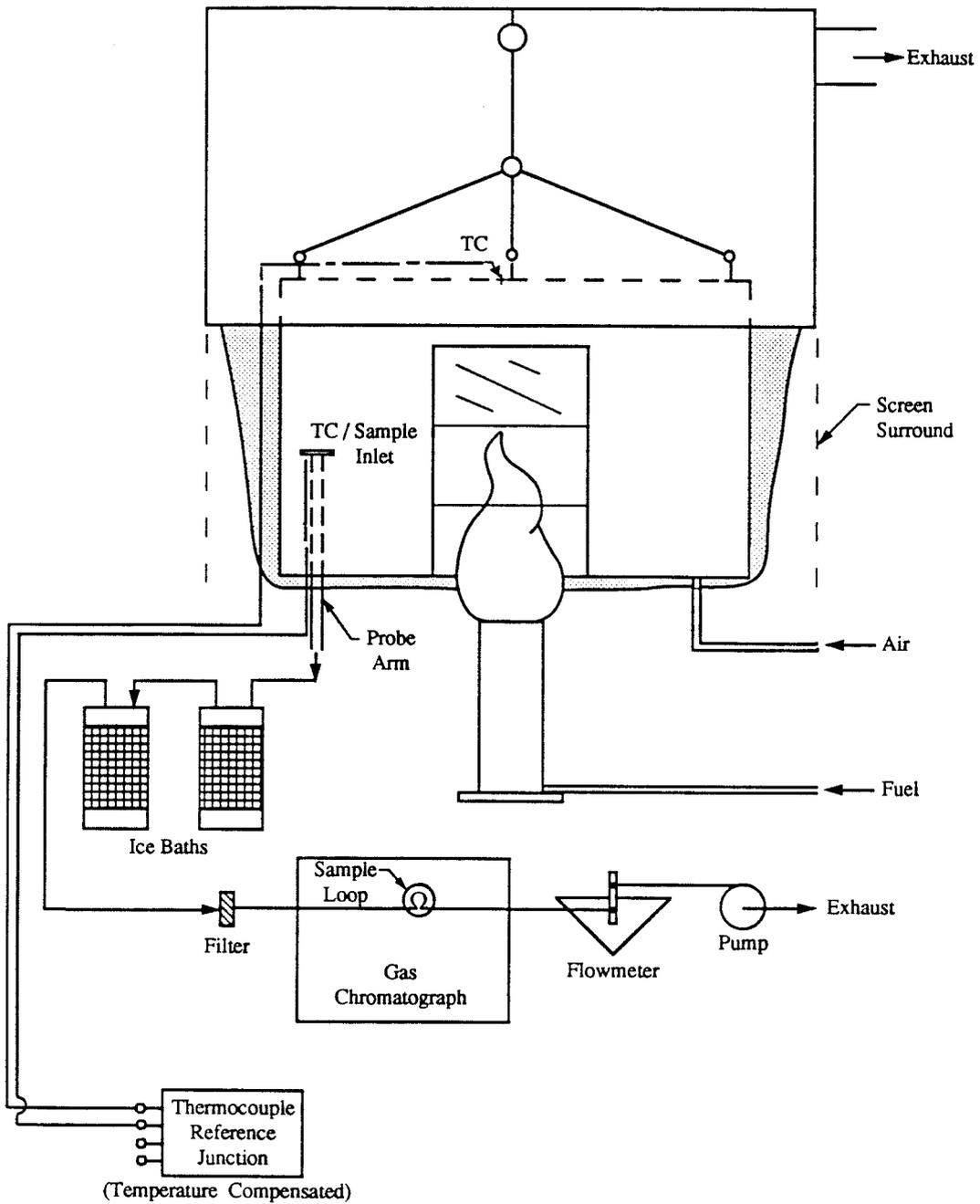
Figure 2.5: Schematic of gas burning and sample analysis facilities
