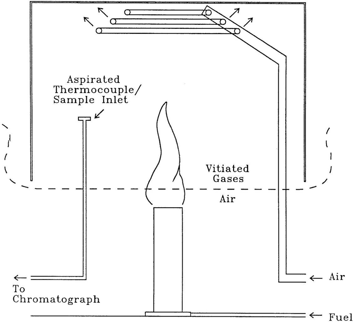
Figure 2.2: Schematic of experimental apparatus with air addition network used in this study
