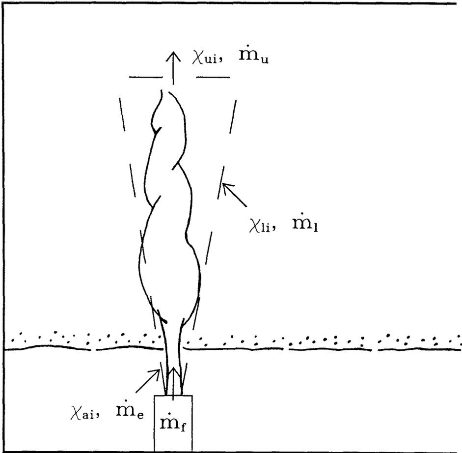
Figure 4.16: Plume reactor model for enclosure fire
