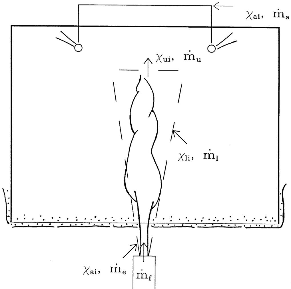
Figure 4.17: Plume reactor model for experiment
